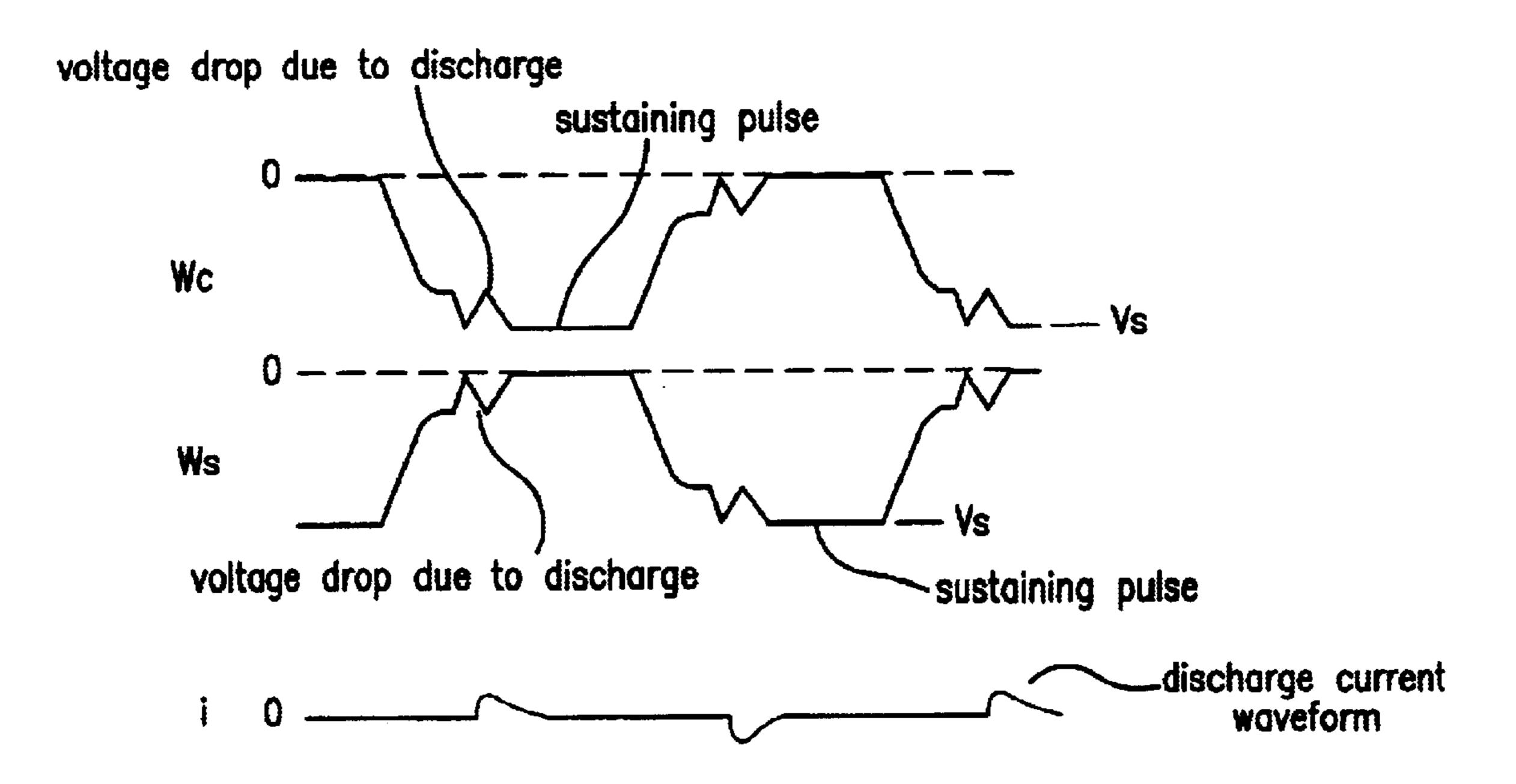
Wc: sustaining electrode driving pulse waveform Ws: scanning electrode driving pulse waveform
