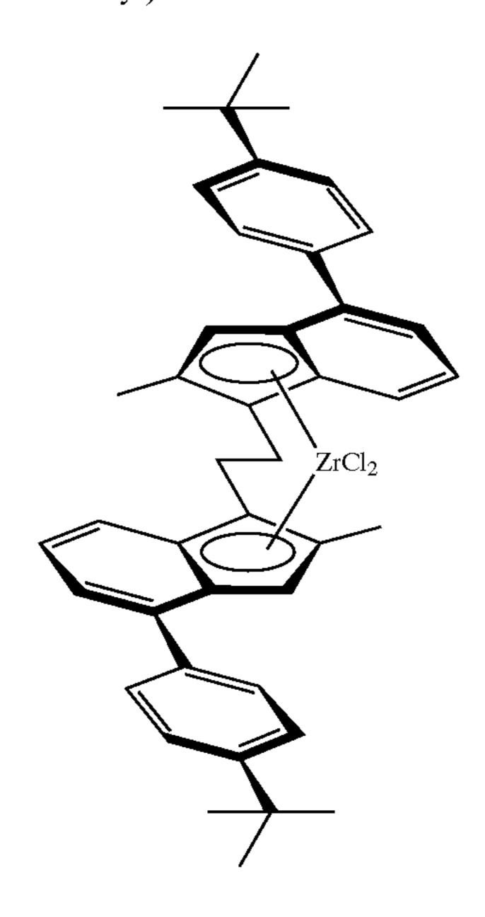
9.1 g (16.5 mmol) of 1,2-bis(2-methyl-4-(4'-tert- 45 butylphenyl)indenyl)ethane and 230 ml of diethyl ether were placed in a 500 ml three-neck flask. The suspension was admixed at room temperature with 20.7 ml (33.1 mmol, 1.6 M in hexane) of n-BuLi.
