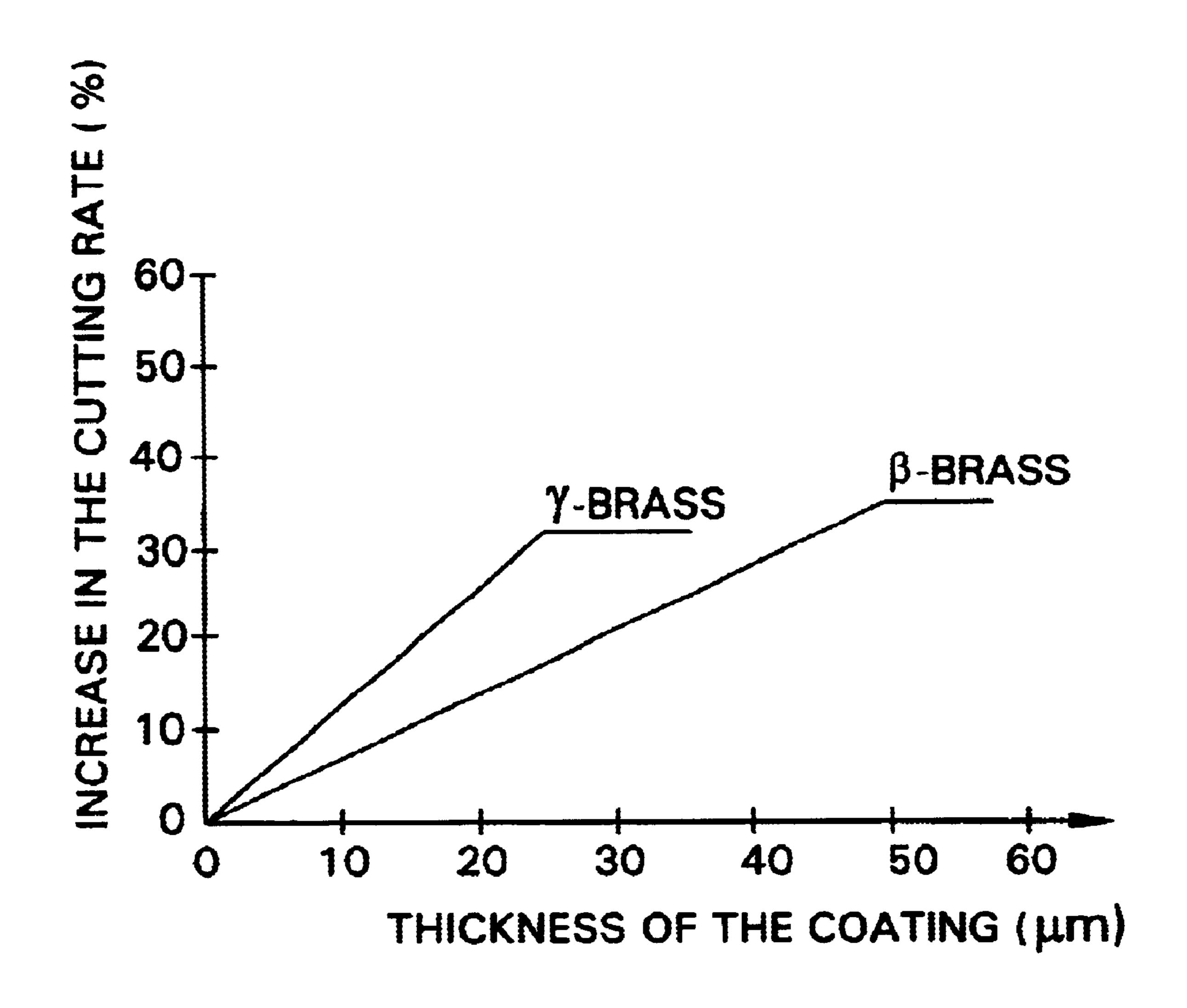
X210Cr12 WORKPIECE MATERIAL: WORKPIECE HEIGHT: 50 mm WIRE DIAMETER: 0.3 mm 12 m/min WIRE RUN-OFF SPEED:
