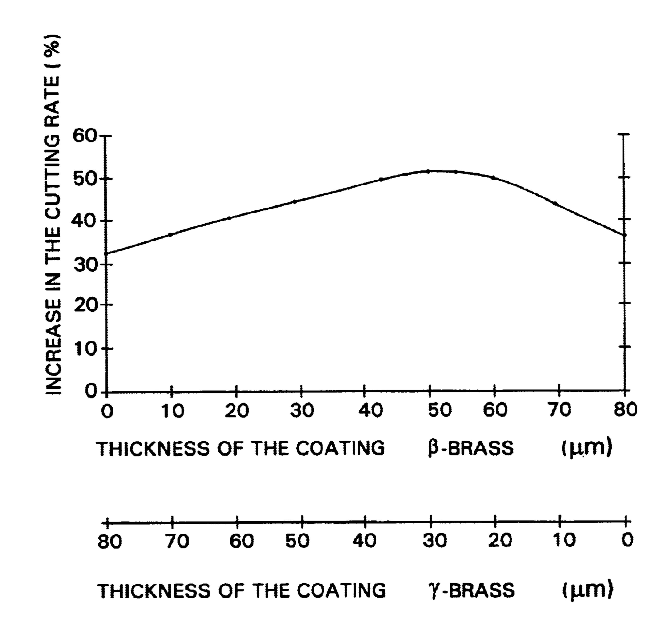
X210Cr12 WORKPIECE MATERIAL: WORKPIECE HEIGHT: 50 mm WIRE DIAMETER: 0.3 mm 12 m/min WIRE RUN-OFF SPEED:
