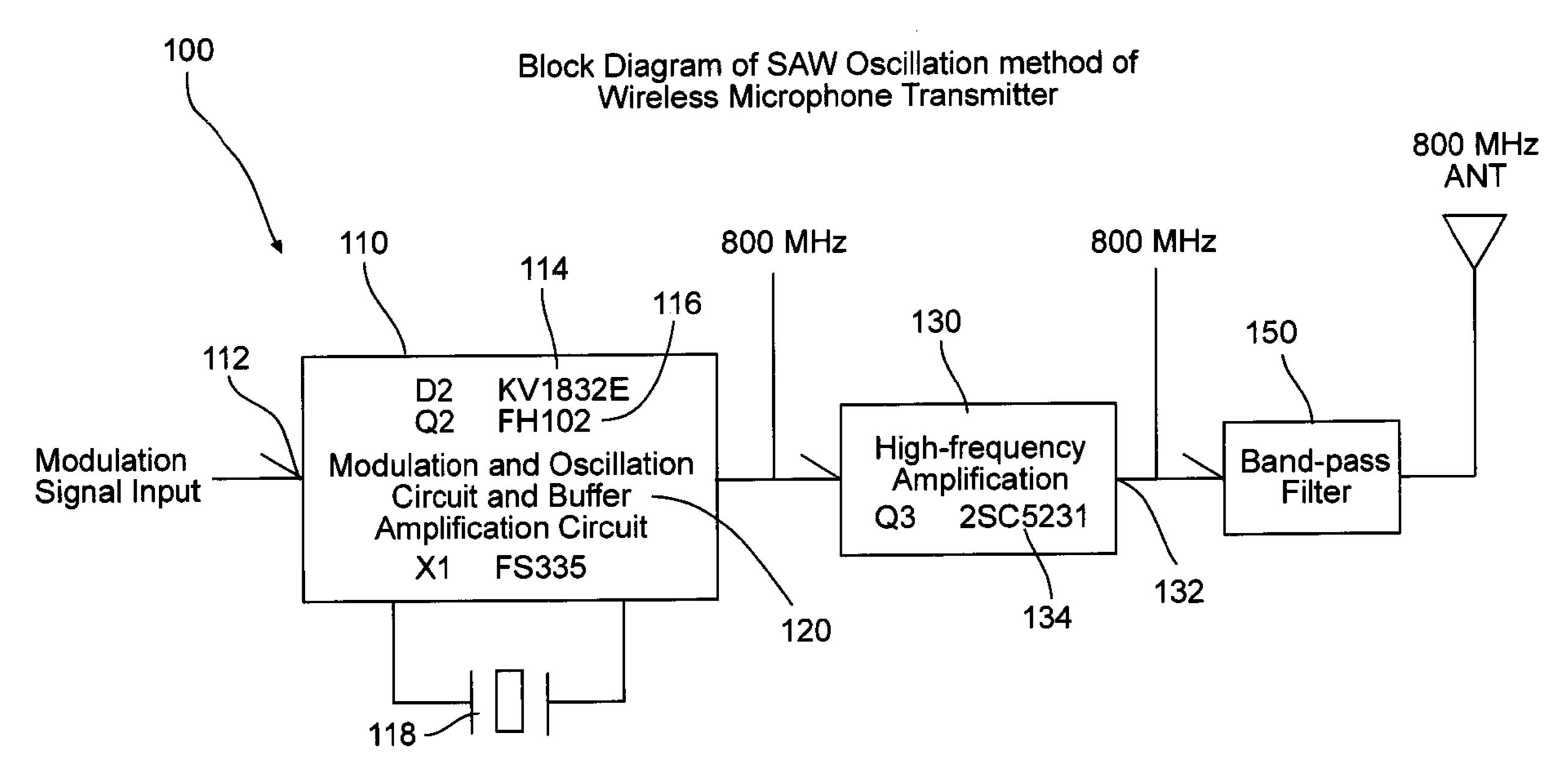
SAW Resonator with Band of 800 MHz
