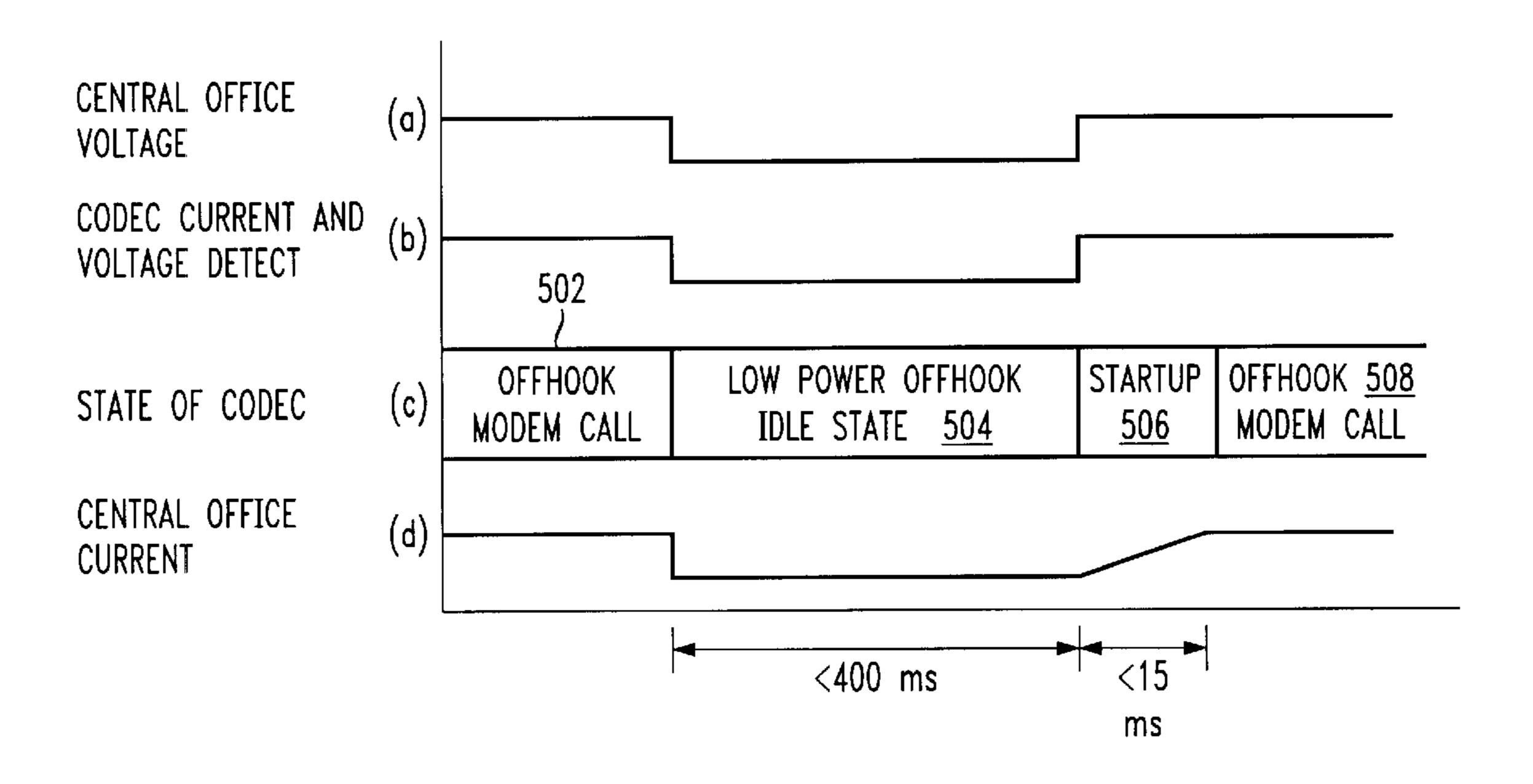
FIG. 6 LOW CURRENT STARTUP TIMING DIAGRAM
