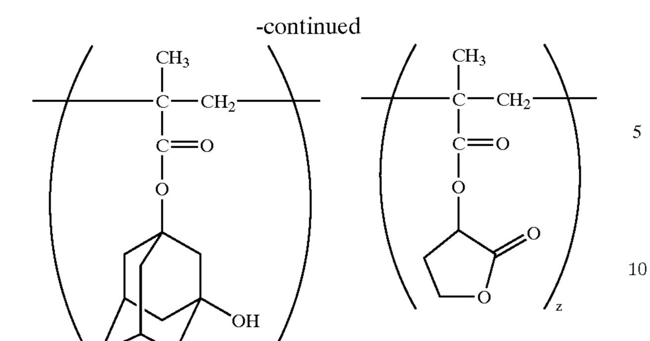
The result of <sup>13</sup>C-NMR measurement showed x:y:z= 31:36:33. The resin had a weight average molecular weight of 10,000.
