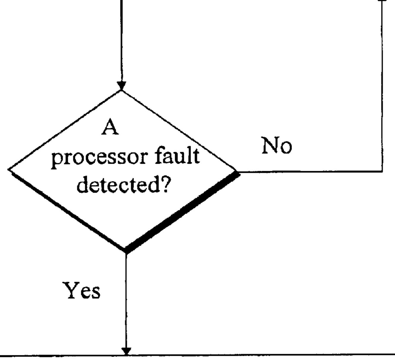
User plane connections within the node relocated from the faulted processor in accordance with the determined priority order in control of a resource handler of the node
