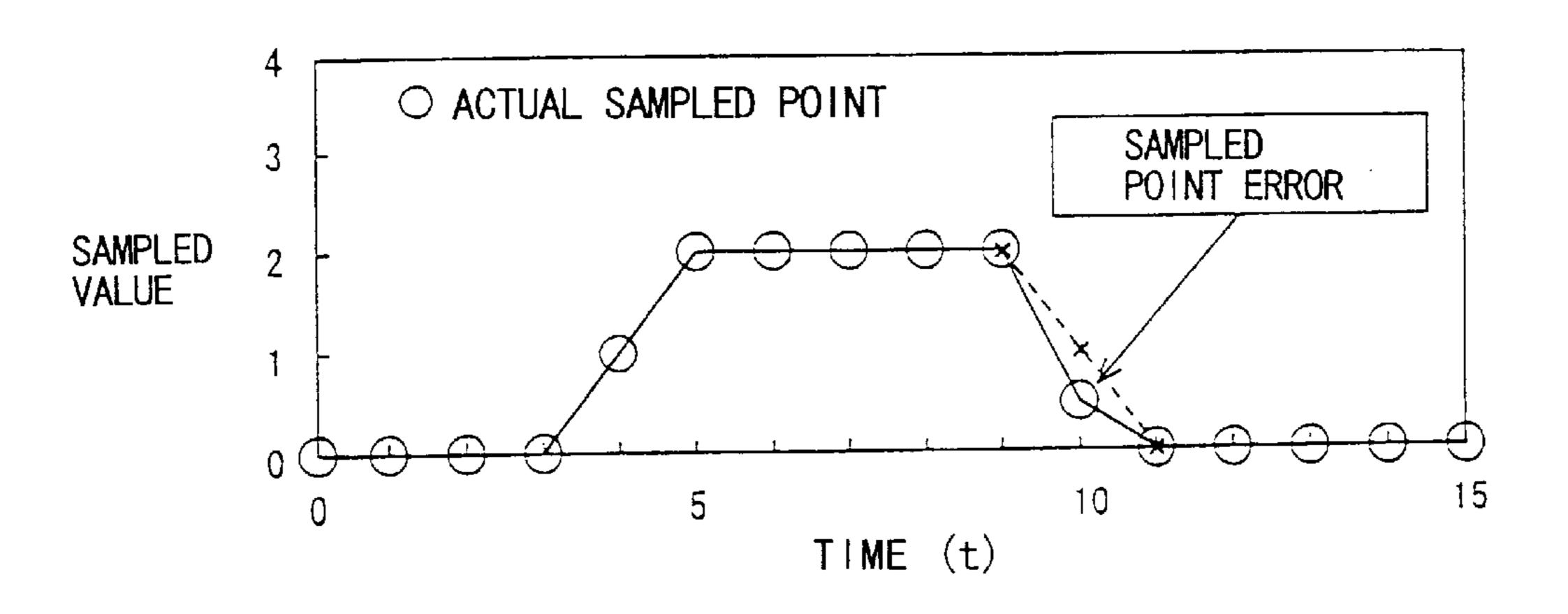
Diagram for illustrating detected data demodulated from the sampled values shown in FIG. 19
