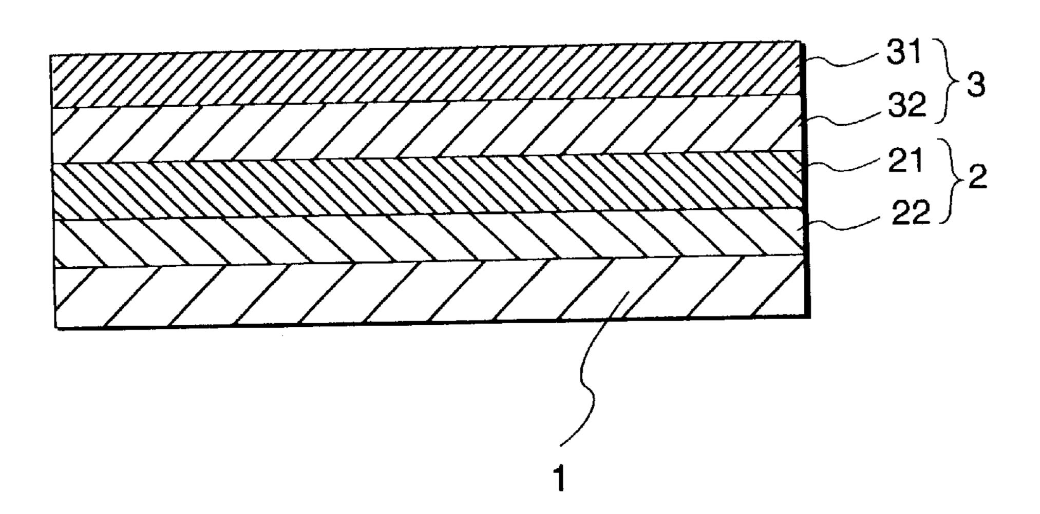
COMPOSITE RETARDER PLATE HAVING RETARDER FILM WITH AT LEAST ONE REFRACTIVE INDEX DIFFERENT FROM THE OTHER INDICES AND A LIQUID CRYSTAL POLYMER PHASE SHEET HAVING A TRANSPARENT LAYER WITH ALL REFRACTIVE INDICES DIFFERENT FROM ONE ANOTHER
