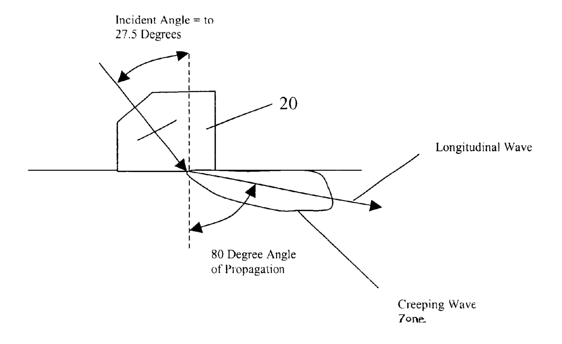
Figure 4: Creeping wave transducer
