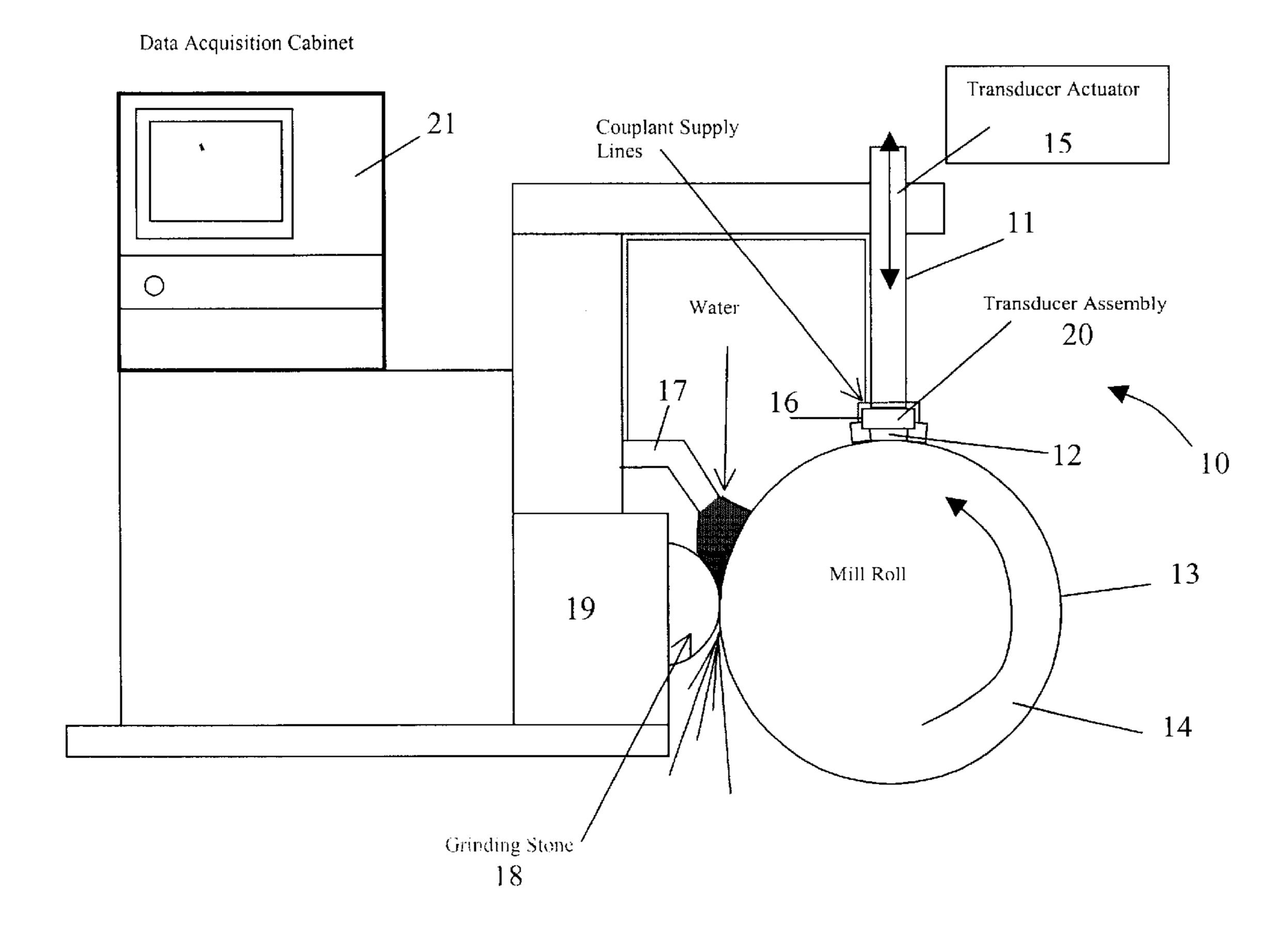
Figure 3: Roll grinding machine with creeping wave inspection system
