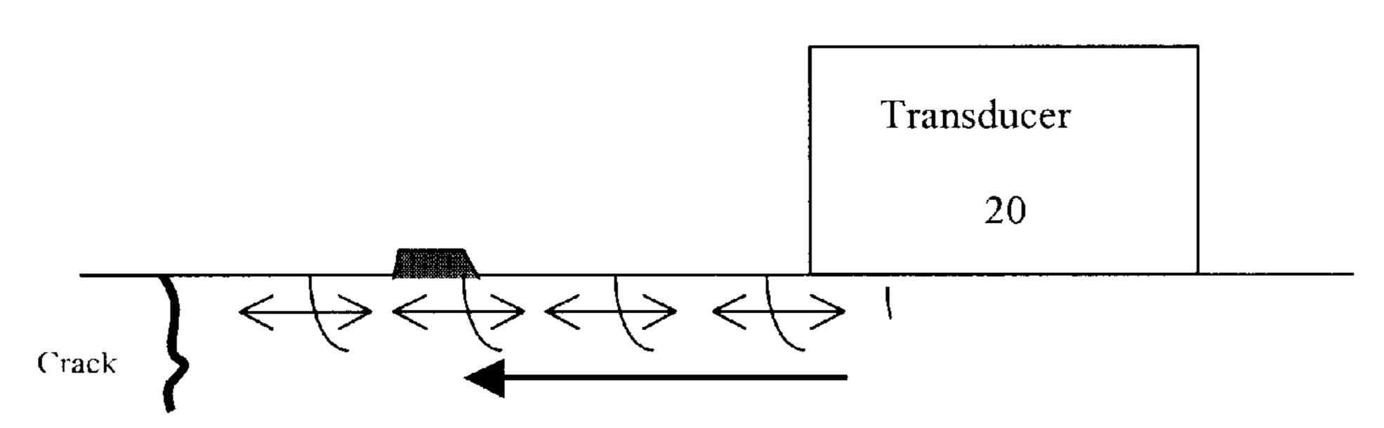
Direction of creeping wave propagation
