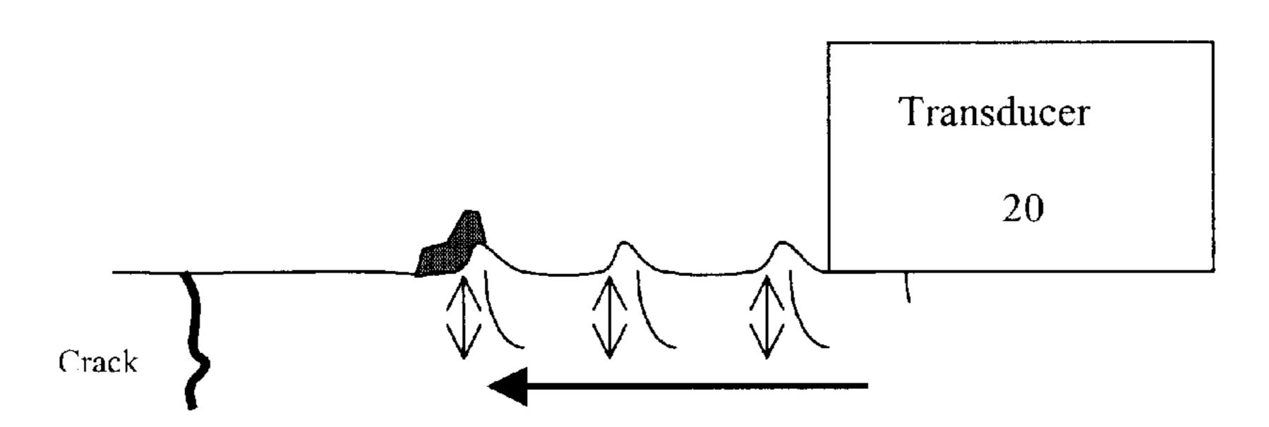
Direction of Surface wave propagation
