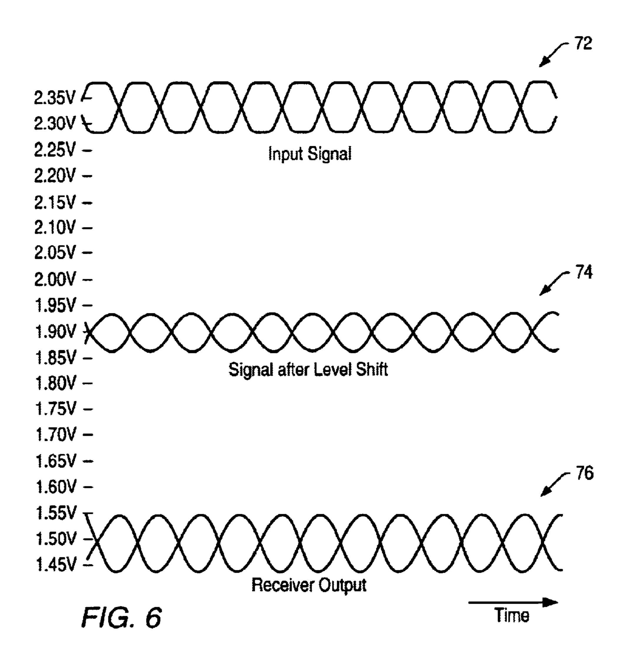
LOW VOLTAGE RECEIVER CIRCUIT AND METHOD FOR SHIFTING THE DIFFERENTIAL INPUT SIGNALS OF THE RECEIVER DEPENDING ON A COMMON MODE VOLTAGE OF THE INPUT SIGNALS
