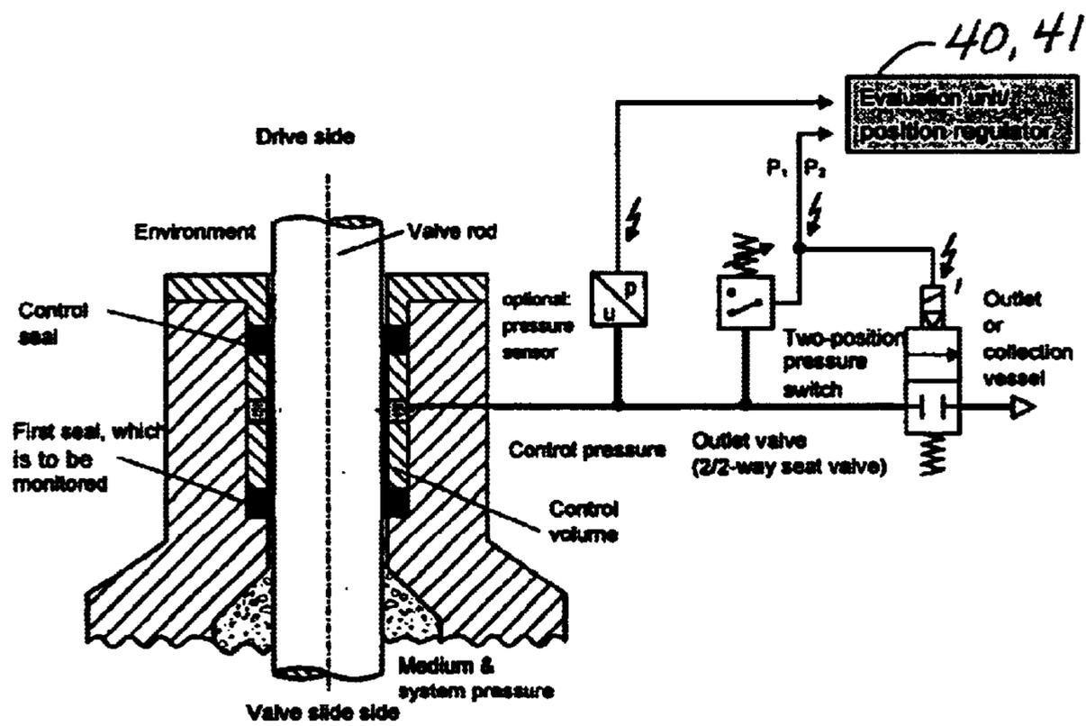
*Figure 4: Monitoring of a seal by observing the control pressure, venting from time to time via a 2/2-way switching valve of the "normally closed" type, driving for example by means of two-position pressure switch*
