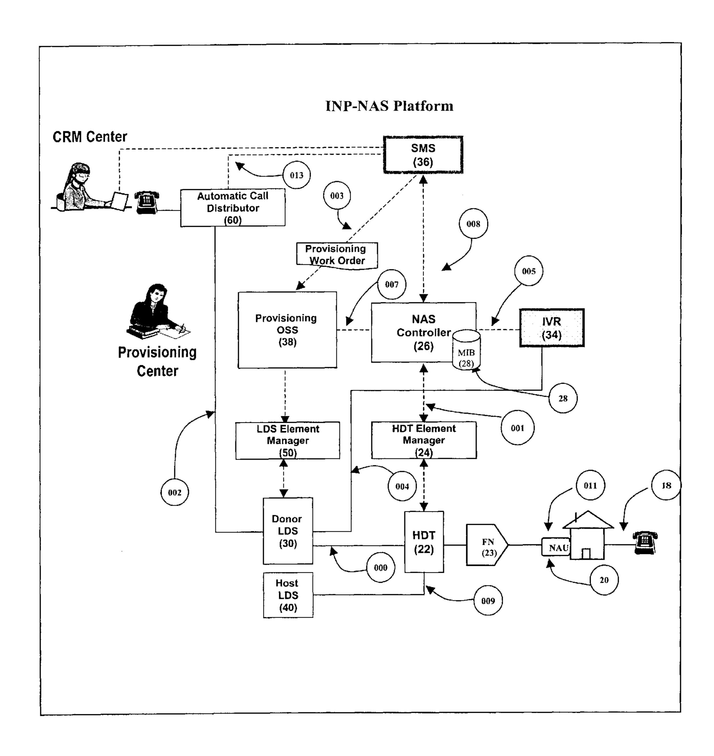
Figure 1 INP Network Access Services Platform Architecture
