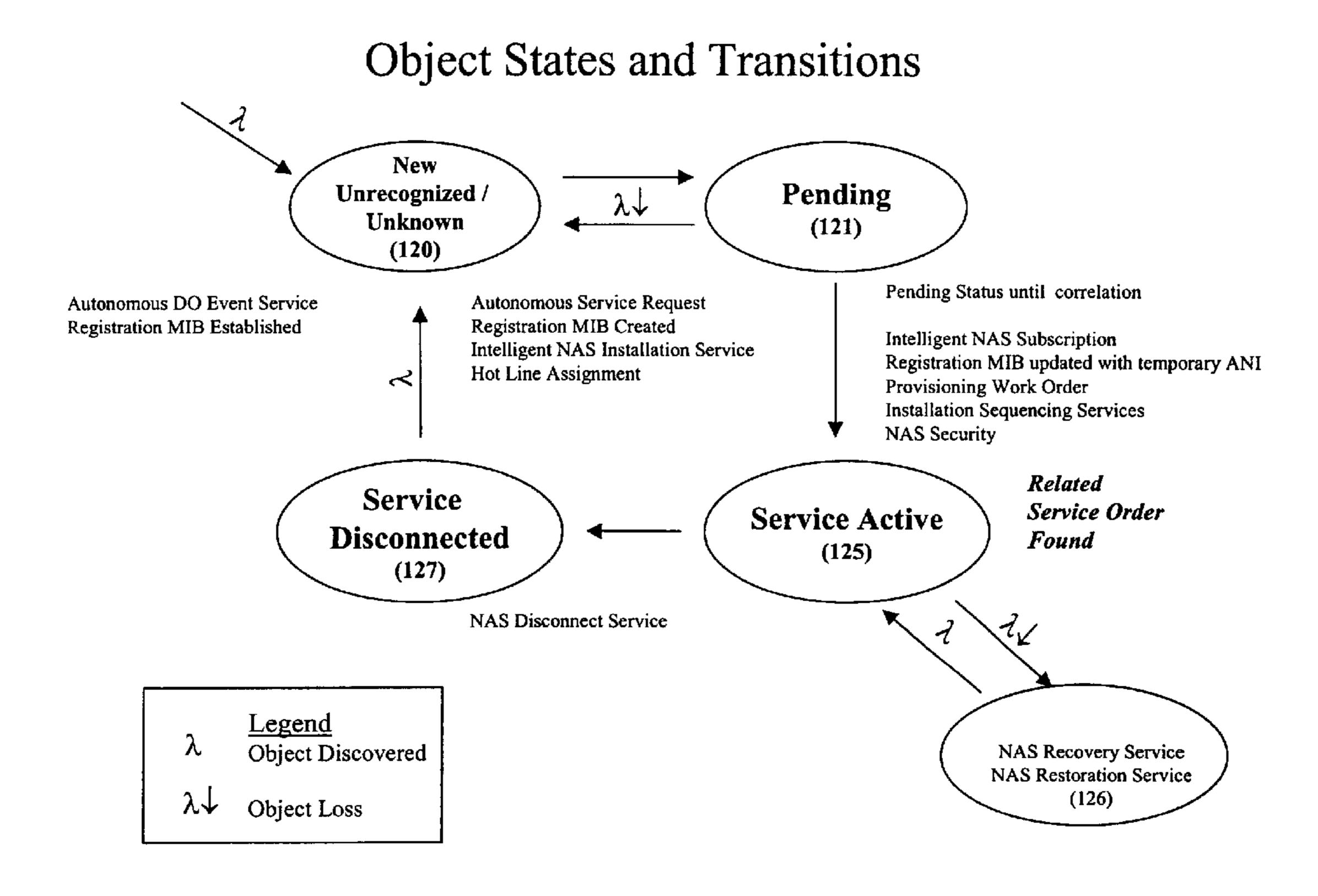
Figure 12 – Events and Services Relationship to Object State Diagram
