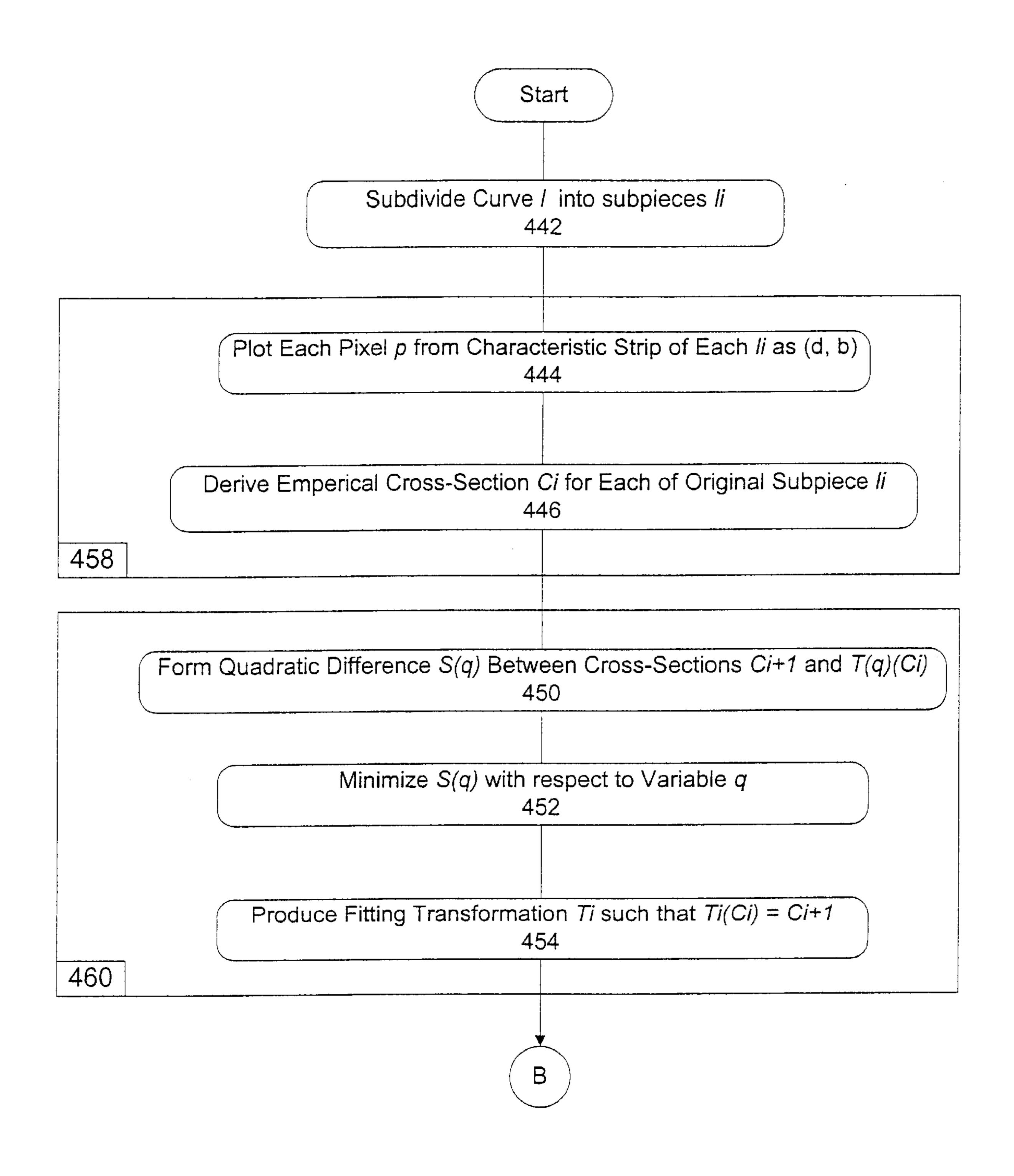
FIG. 24a General Plotting Procedure
