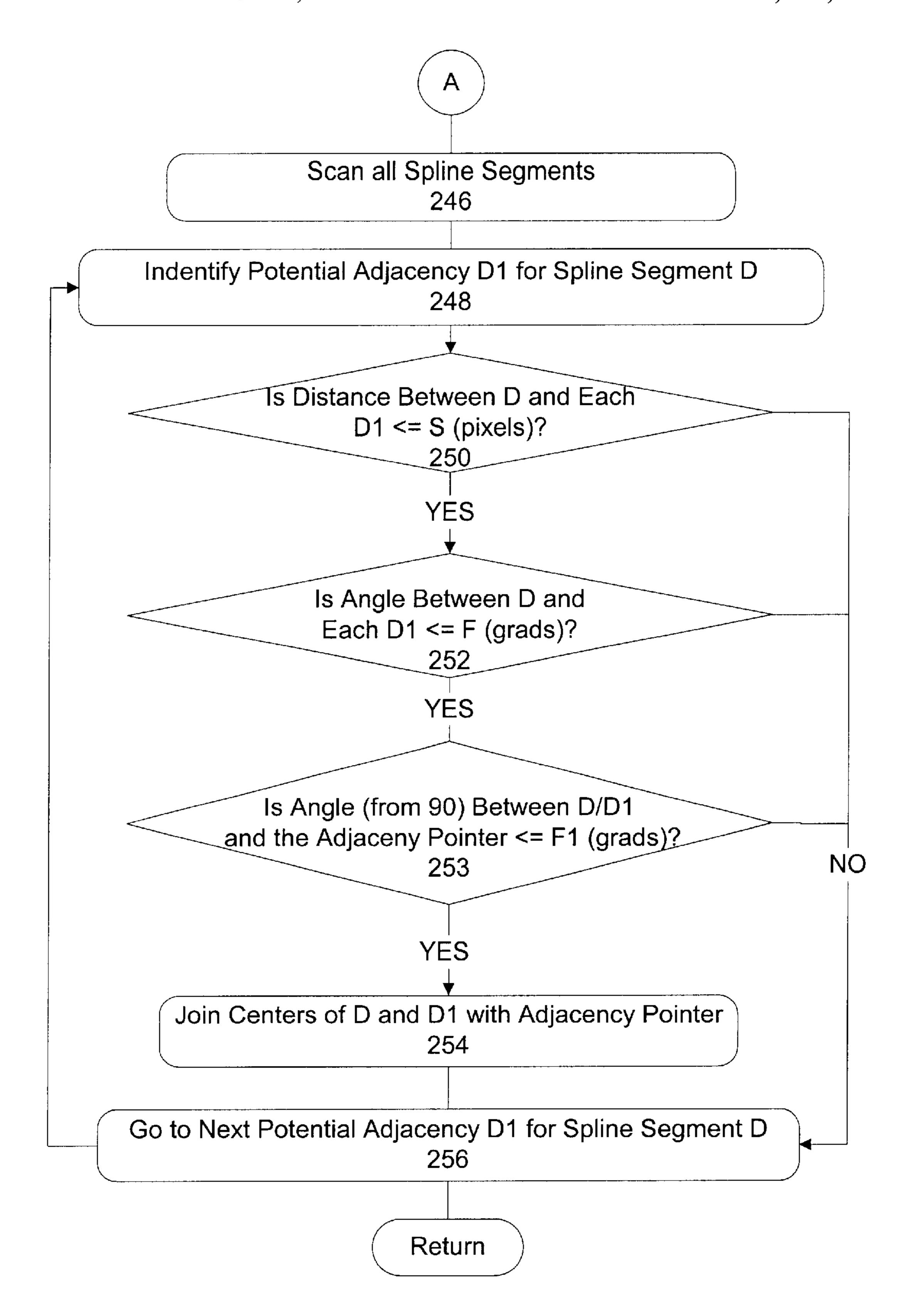
FIG. 16 Adjacency Detection
