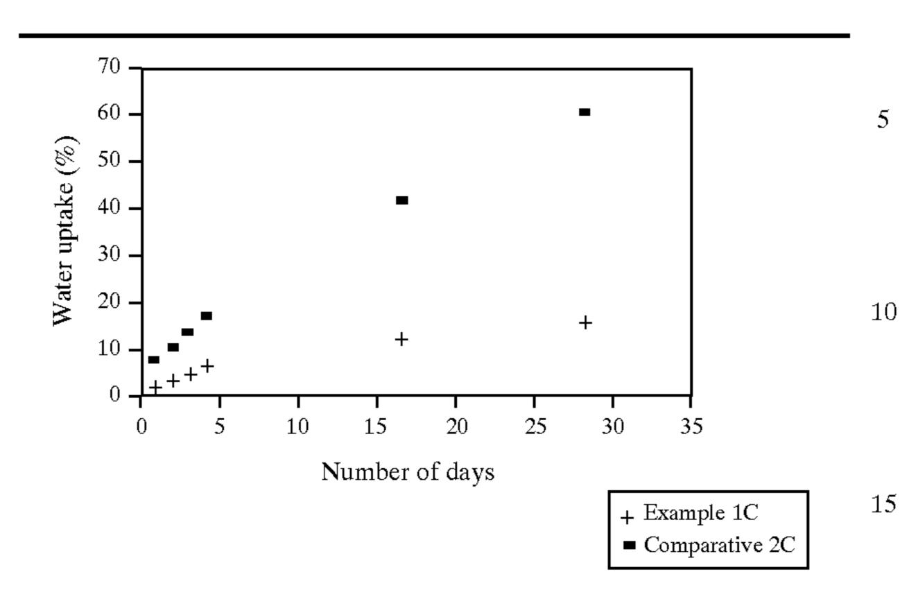
Example 1C and Comparative Example 2C show that the use of a reactive surfactant corresponding to the claimed formula (I) makes it possible to reduce the water uptake of the latice films by a factor of 4.
