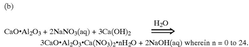
The presence NaOH does not appear to interfere with sequestration of chloride or with the action of nitrite on steel and, as a result, it is not necessary to remove the NaOH by washing the product compounds. Alternatively, the  $3\text{CaO}\cdot\text{Al}_2\text{O}_3\cdot\text{Ca}(\text{NO}_3)_2\cdot n\text{H}_2\text{O}$  and  $\text{Ca}(\text{NO}_3)_2$  can be crystallized from the NaOH solution.
