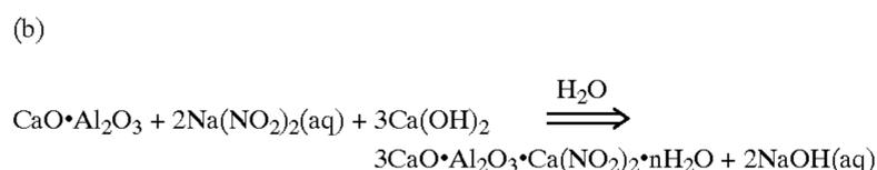
The presence NaOH does not appear to interfere with sequestration of chloride or with the action of nitrite on steel and, as a result, it is not necessary to remove the NaOH by washing the product compounds. Alternatively, the
