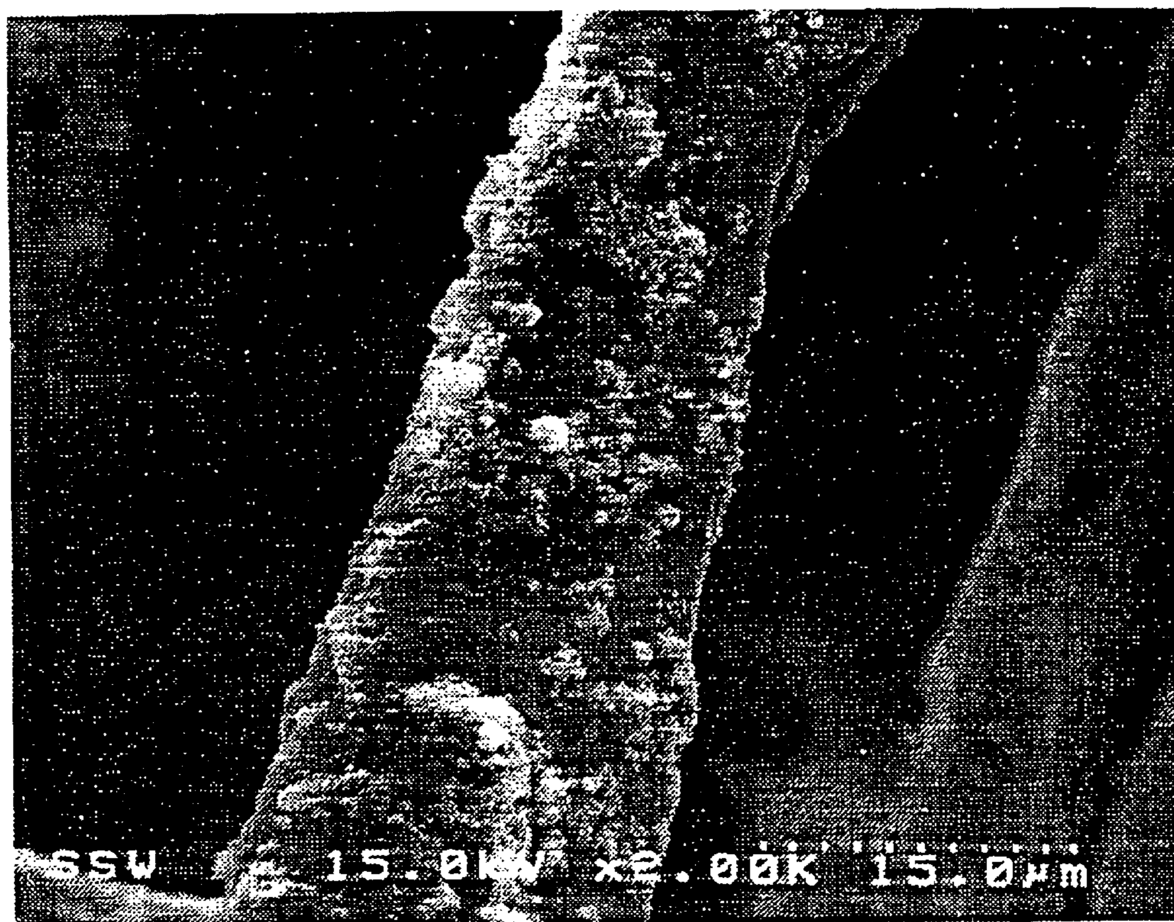
Figure 7 : Close up picture of Figure 5.5 showing a single treated strand and TiO 2 attached to it firmly.
