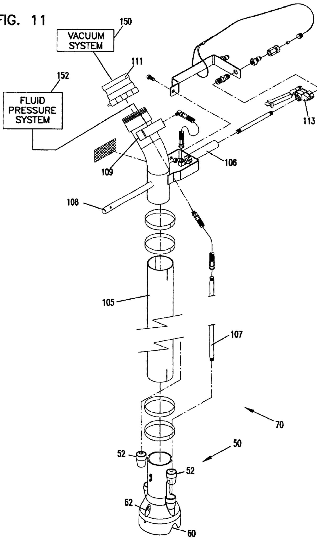
**NOZZLE MOUNT FOR SOFT EXCAVATION****CROSS-REFERENCE TO RELATED APPLICATIONS**
