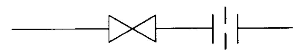
Valve plug drilled with fixed restriction when closed and minimal restriction when open.
