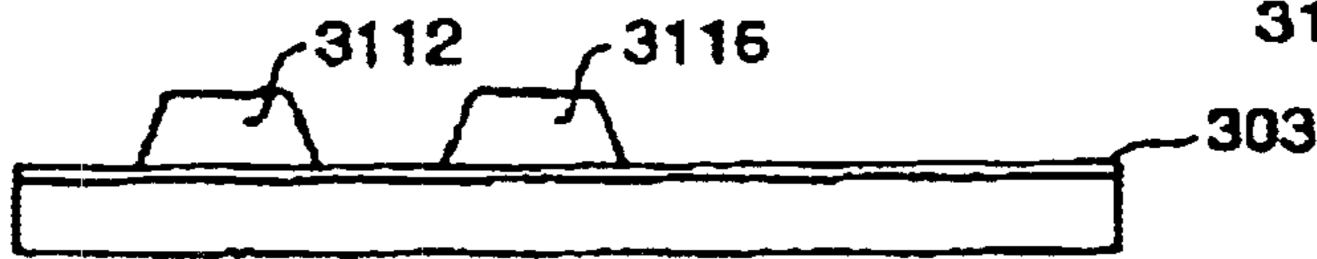
Fig. 15c PATTERNING OF FIRST METAL FILM
