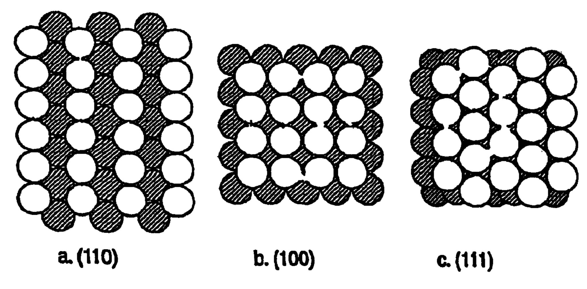
SURFACE STRUCTURE OF DIFFERENT Pd CRYSTAL PHASES
