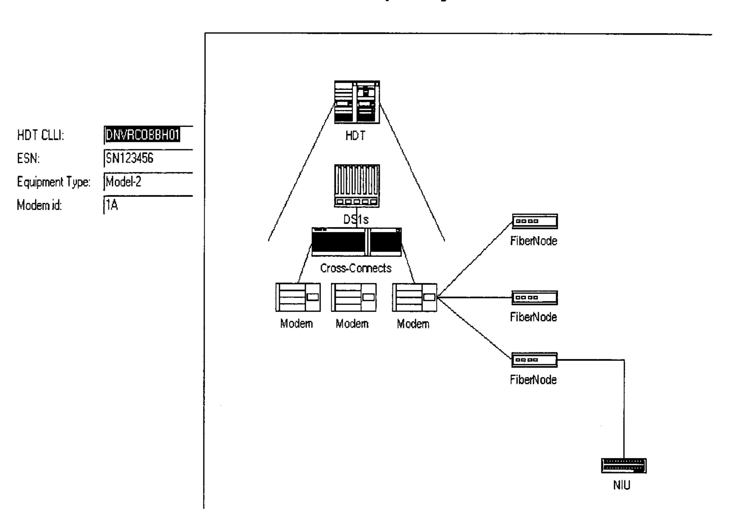
Figure 7 – Object Discovery message arriving from HDT upon the event that an NAU was powered up on the CATV network.
