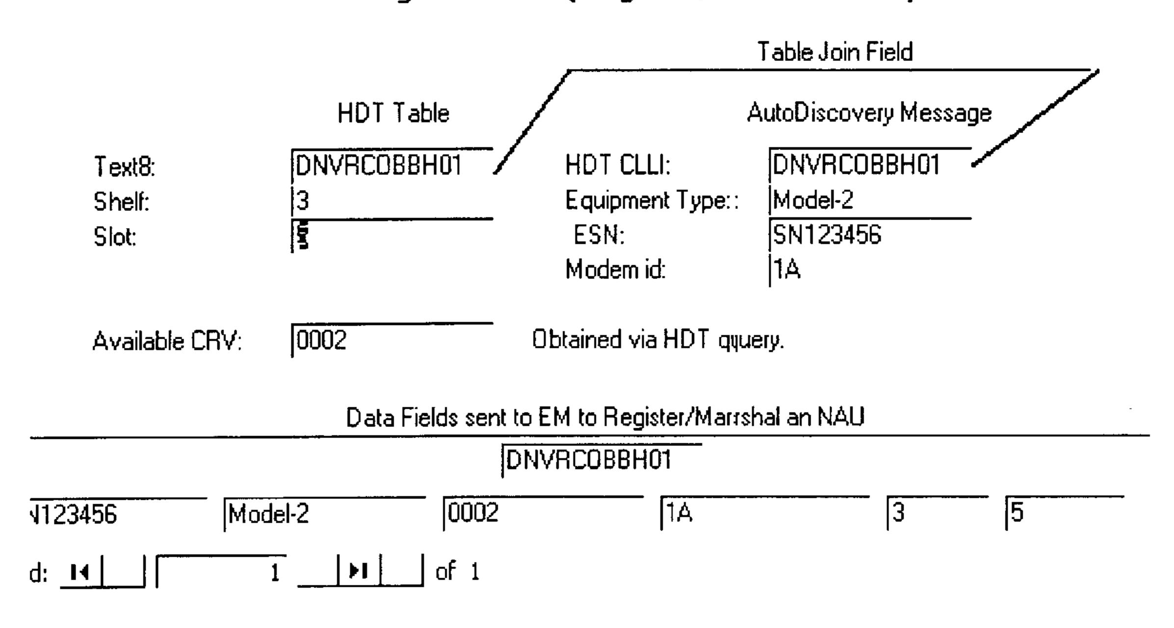
Figure 8 – Matching the Object Discovery Message to the static HDT information.
