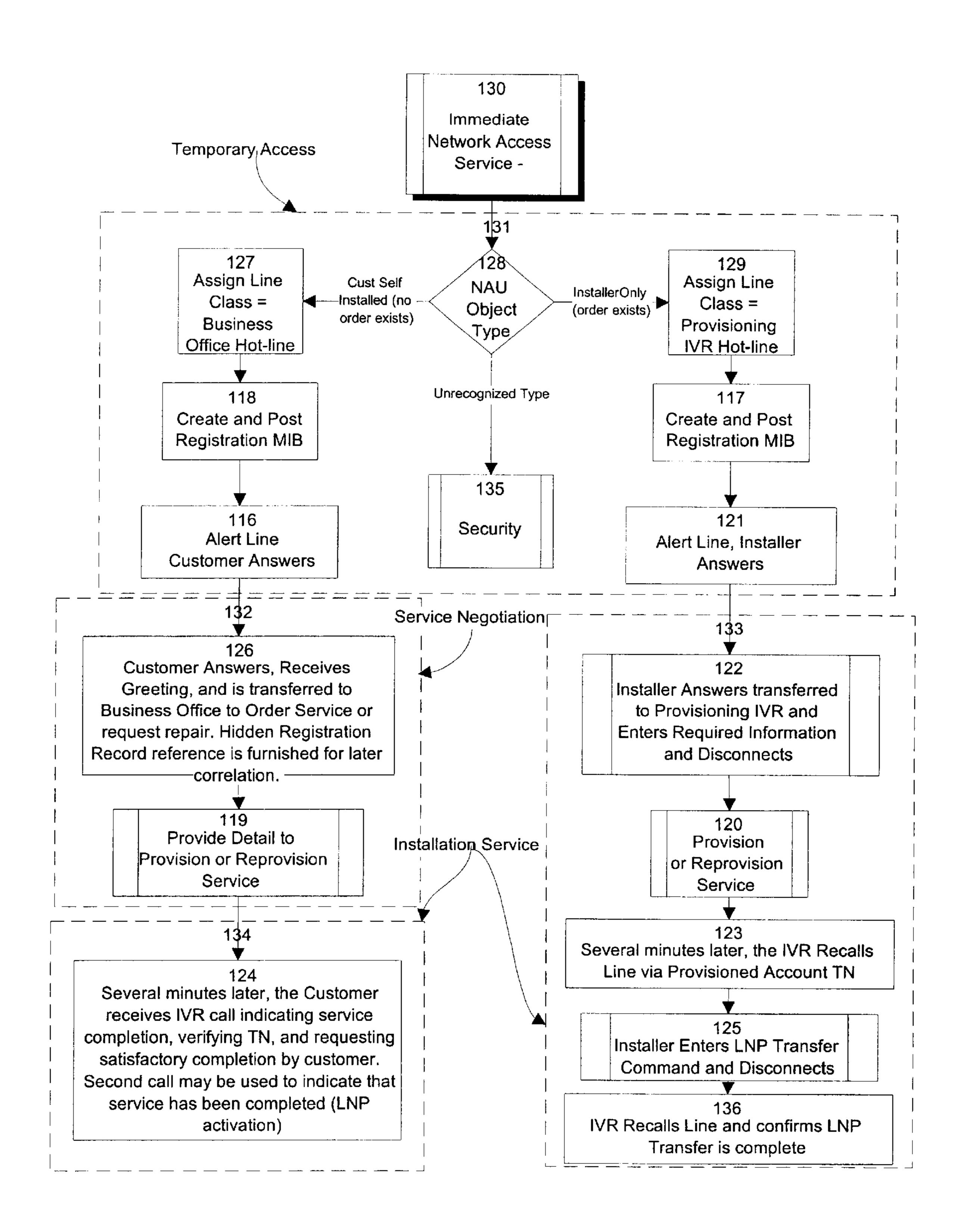
Figure 3 Immediate Network Access Service
