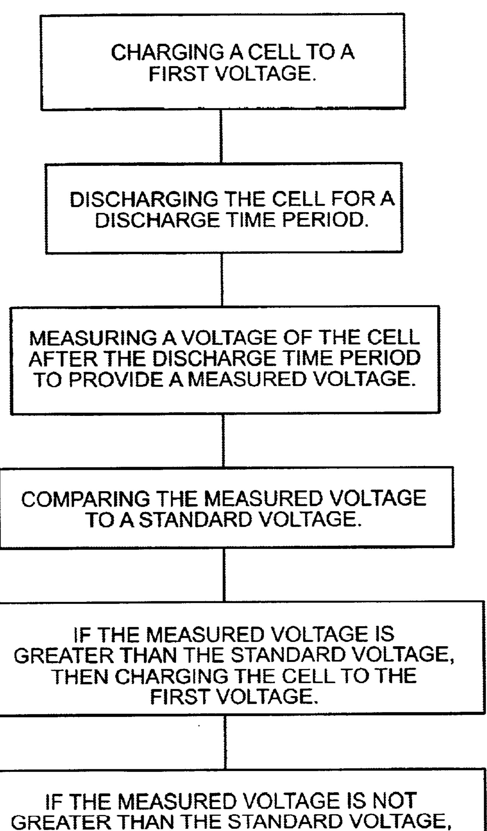
IF THE MEASURED VOLTAGE IS NOT GREATER THAN THE STANDARD VOLTAGE, THEN CHARGING THE CELL TO A SECOND VOLTAGE.
