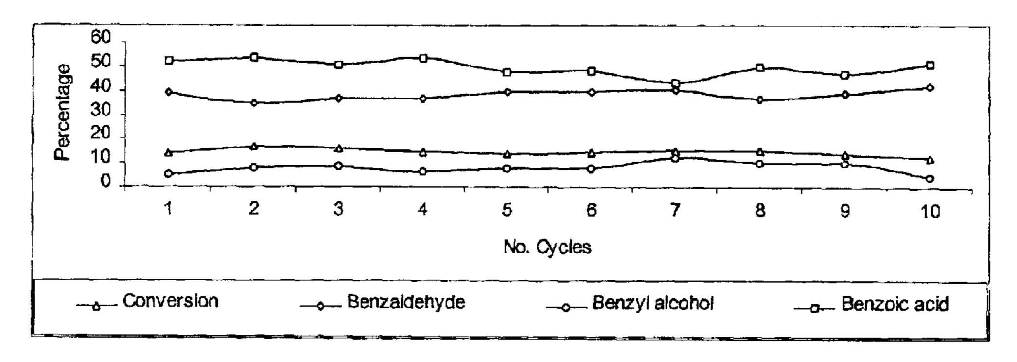
Reaction Volume: 200 ml; Toluene: 64.32 w/v%; Cobalt acetate: 0.01 gmol/L; Manganese acetate: 0.0008 gmol/L; Sodium bromide: 0.0036gmol/L; Time: 1 h; Temperature: 120°C; Pressure: 10 bar; Air flow: 2 L/min.
