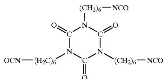
The water-modified fluorochemical carbamates are typically prepared by first charging the polyisocyanate, the perfluoroalkyl compound and a dry organic solvent such as
