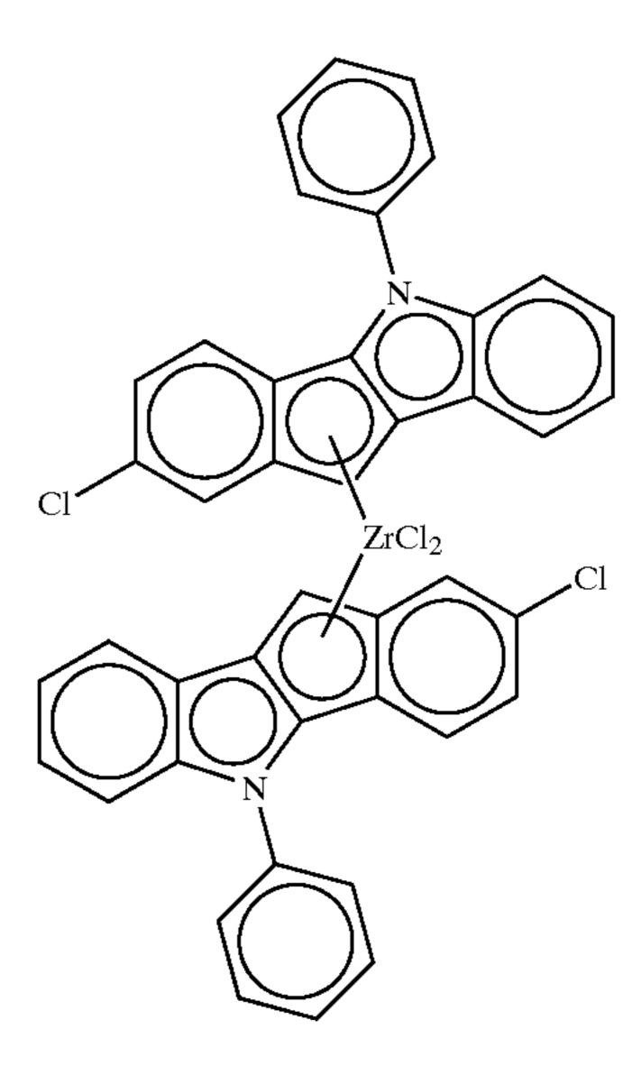
and an alumoxane activator; wherein the resulting copolymer has isotactic and atactic stereoblock sequences.
