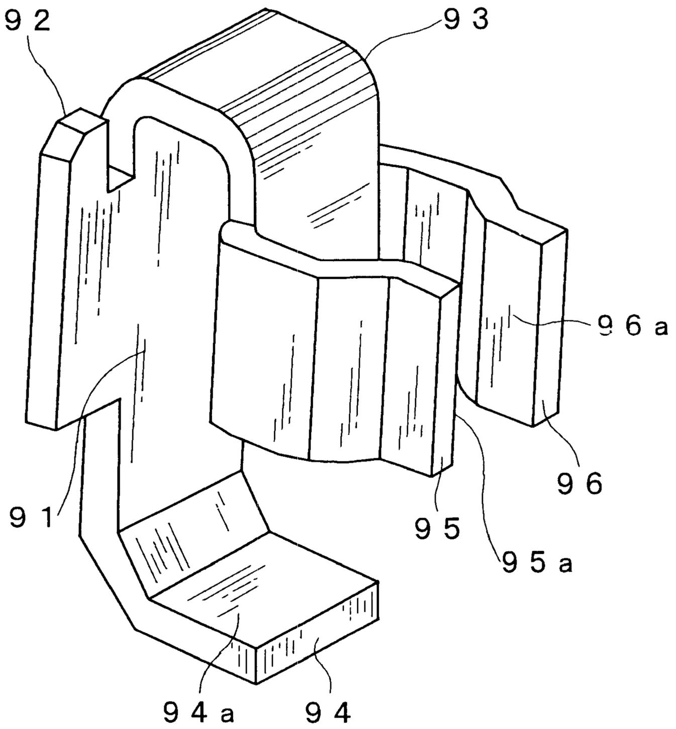
**CONTACT FOR PGA AND PGA SOCKET****BACKGROUND OF THE INVENTION**
