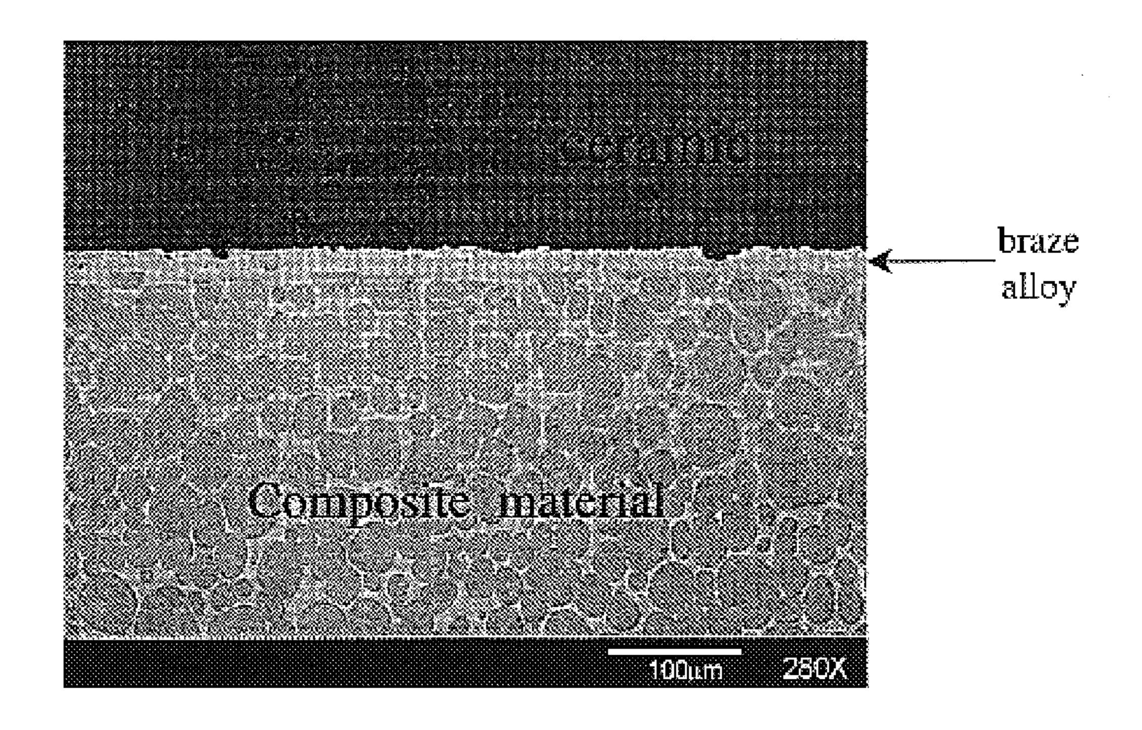
Figure 2. Cross-section of Al<sub>2</sub>O<sub>3</sub> joined to composite.
