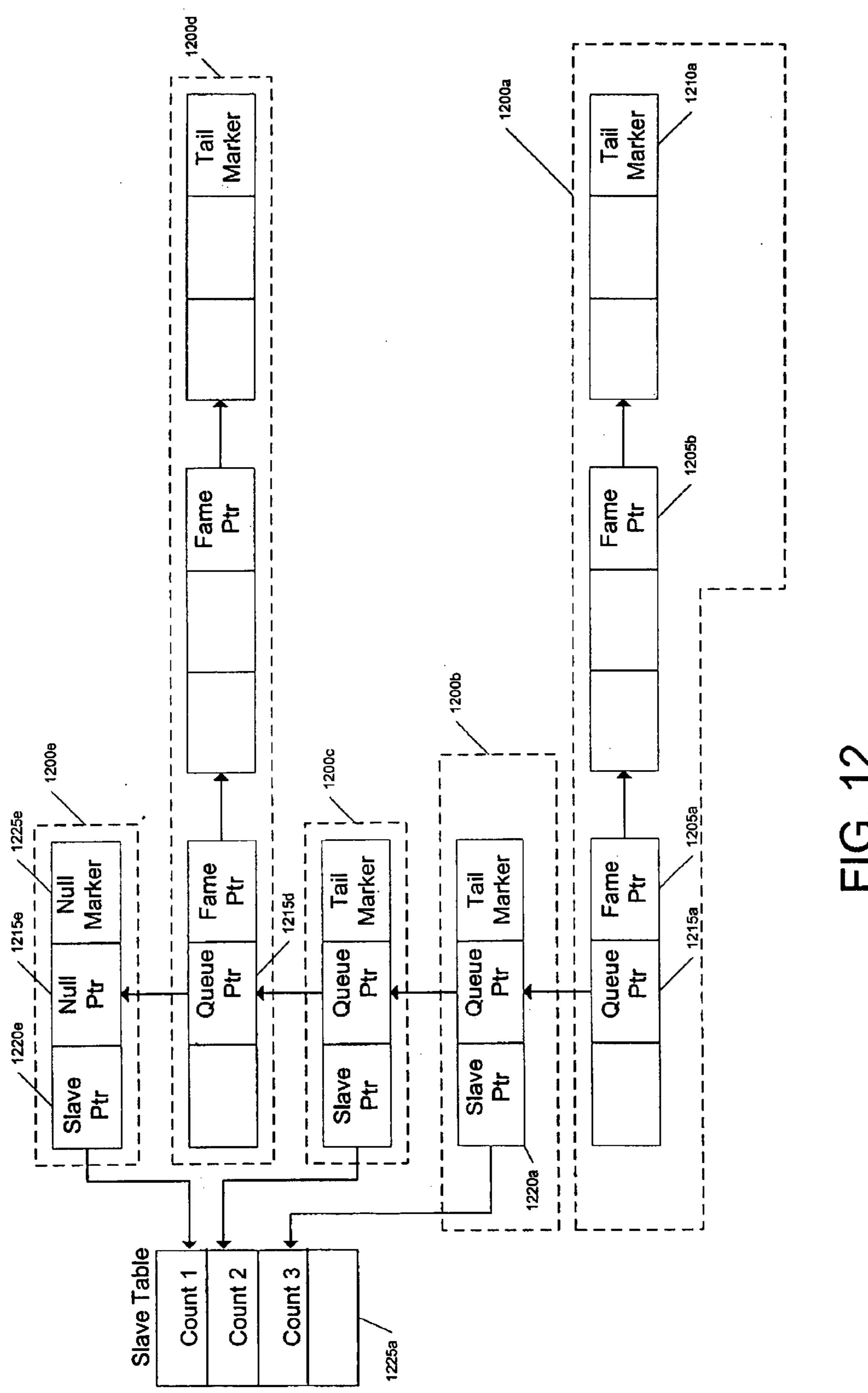
METHODS, SWITCHES, SYSTEMS, AND COMPUTER PROGRAM PRODUCTS FOR FAIR TRANSMISSION OF DATA RECEIVED AT MULTIPLE INPUTS IN THE ORDER RECEIVED IN A QUEUED MEMORY SWITCH
