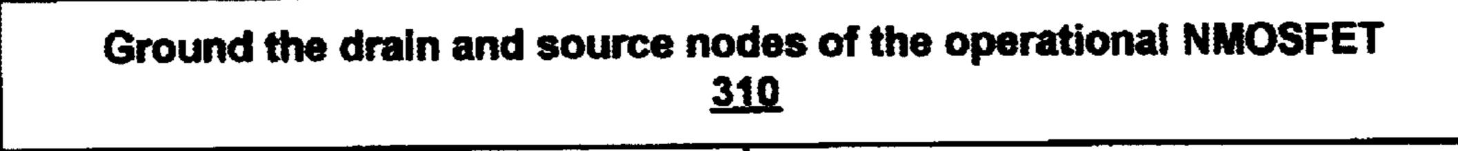
Apply a range of voltages at the gate node and measure the gate direct tunneling current at each applied voltage
