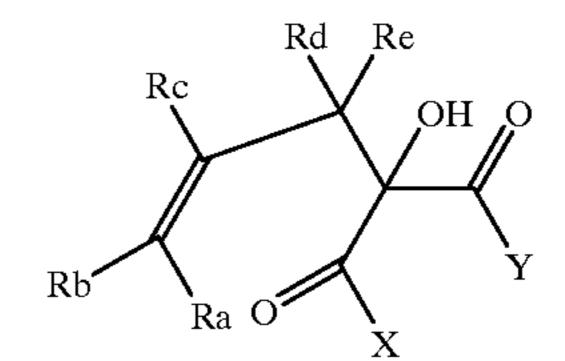
wherein  $R_a$ ,  $R_b$ ,  $R_c$ ,  $R_d$  and  $R_e$  are independently selected from the group consisting of H, alkyl groups and substituted alkyl groups having about 1 to  $10^6$  carbon atoms, alkenyl groups and substituted alkenyl groups having about 3 to  $10^6$  carbon atoms, wherein the substituents on the alkyl and/or alkenyl groups are selected from the group consisting of alkoxy, halogen, CN, OH,  $HO(CH_2CH_2O)_x$  (X=1-10), acyl, acyloxy and aryl substituents.
