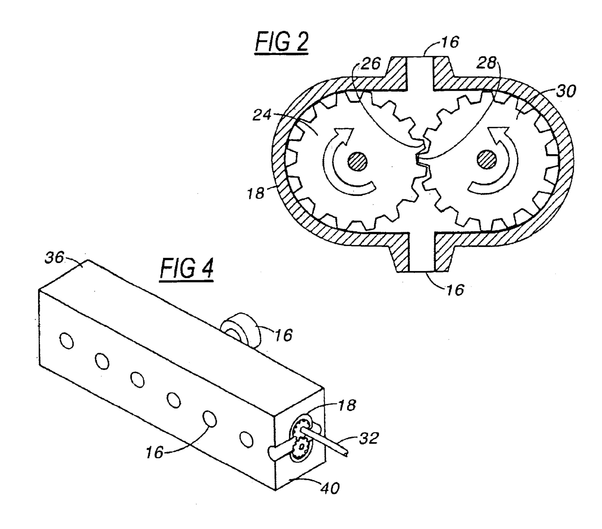
METHOD FOR EMPLOYING A GEAR PUMP WITH AN INJECTION MOLDING MACHINE COMPRISING THE STEP OF
