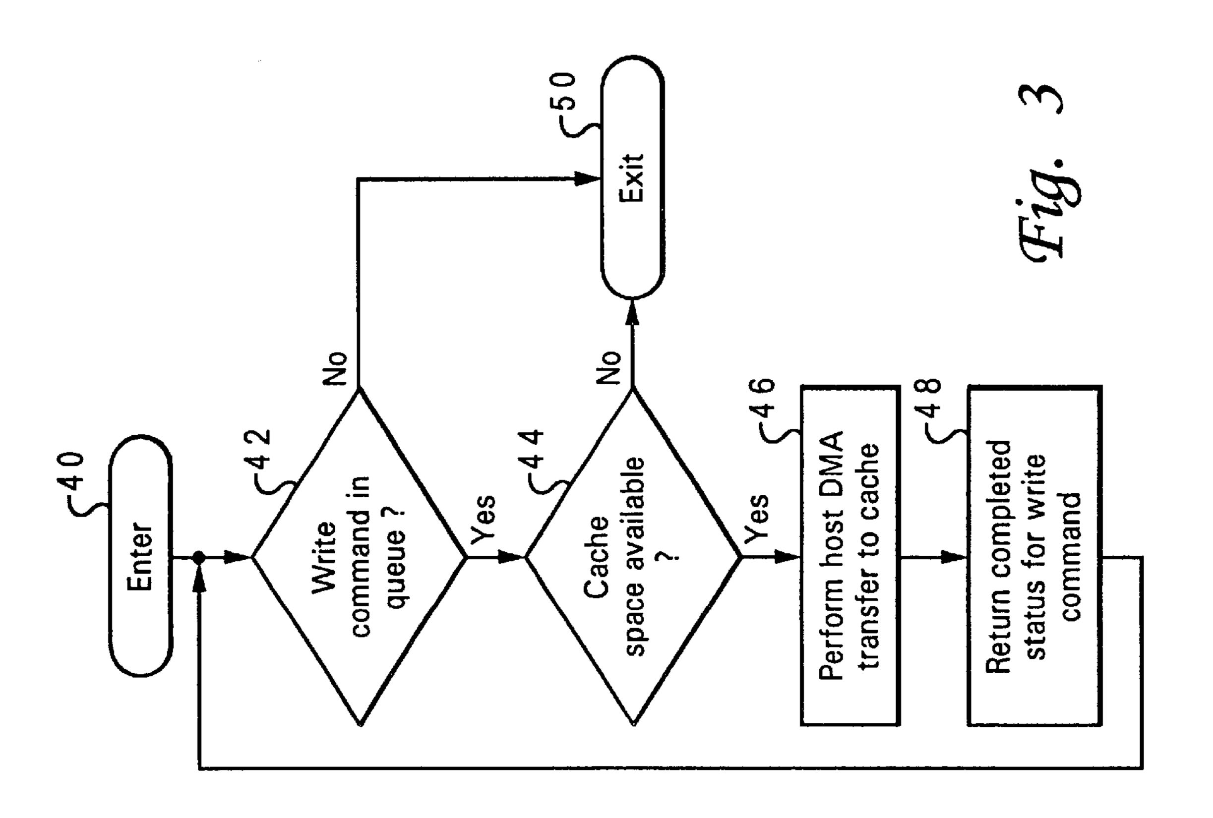
DATA STORAGE DEVICE AND METHOD FOR REDUCING WRITE MISSES BY COMPLETING TRANSFER TO A DUAL-PORT CACHE BEFORE INITIATING A DISK WRITE OF THE DATA FROM THE CACHE
