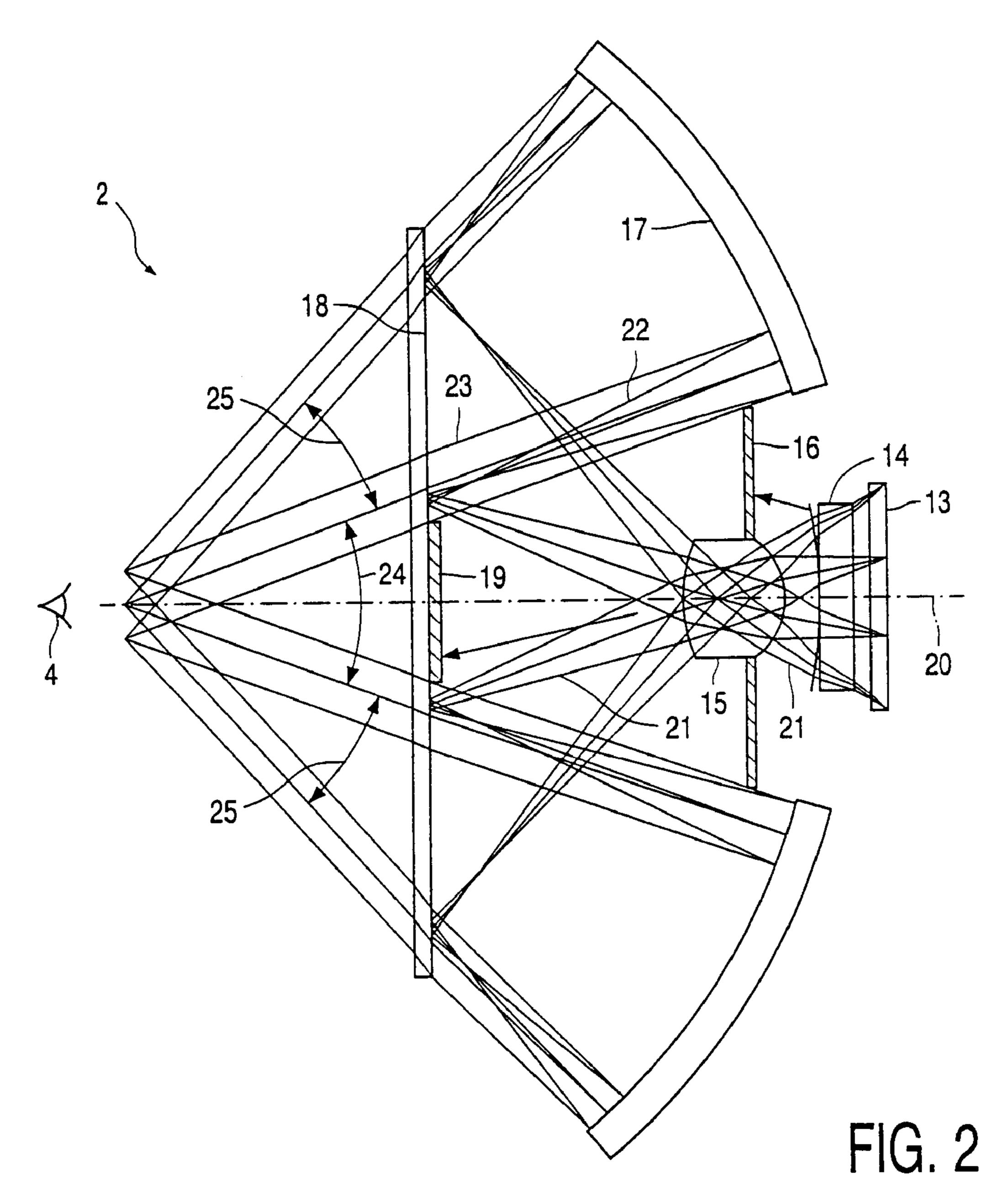
The invention relates to a display device comprising at least one line modulation panel and at least two projection elements, in which, in operation, an image having a relatively high resolution in a relatively small field of view is presented to a first eye by means of the first projection element, while an image having a relatively low resolution in a relatively large field of view is presented to a second eye by means of the second projection element.
