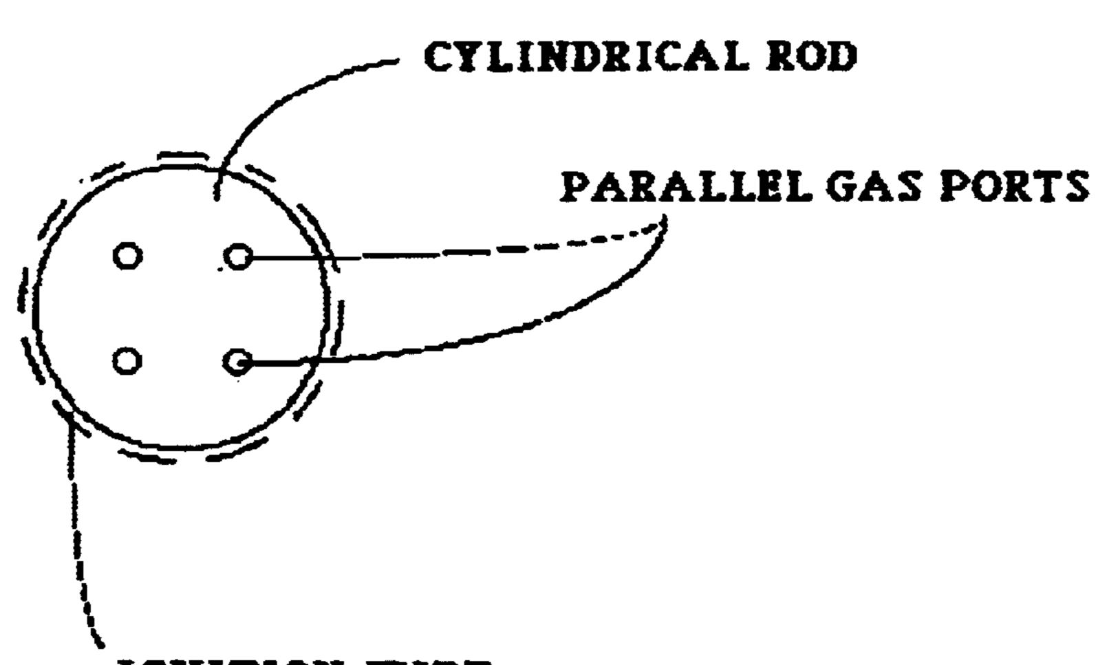
IGNITION WIRE WRAPPED AROUND OUTSIDE OF ROD (COULD ALSO BE COVERED OR COATED BY CERAMIC)
