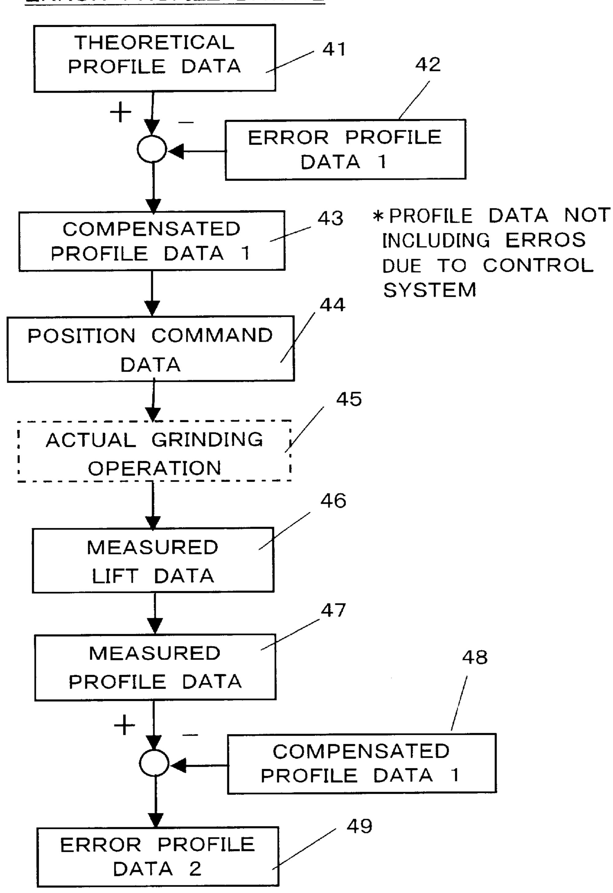
\*ERROR INFORMATION DUE TO MECHANICAL SYSTEM AND TOOL IS SET.
