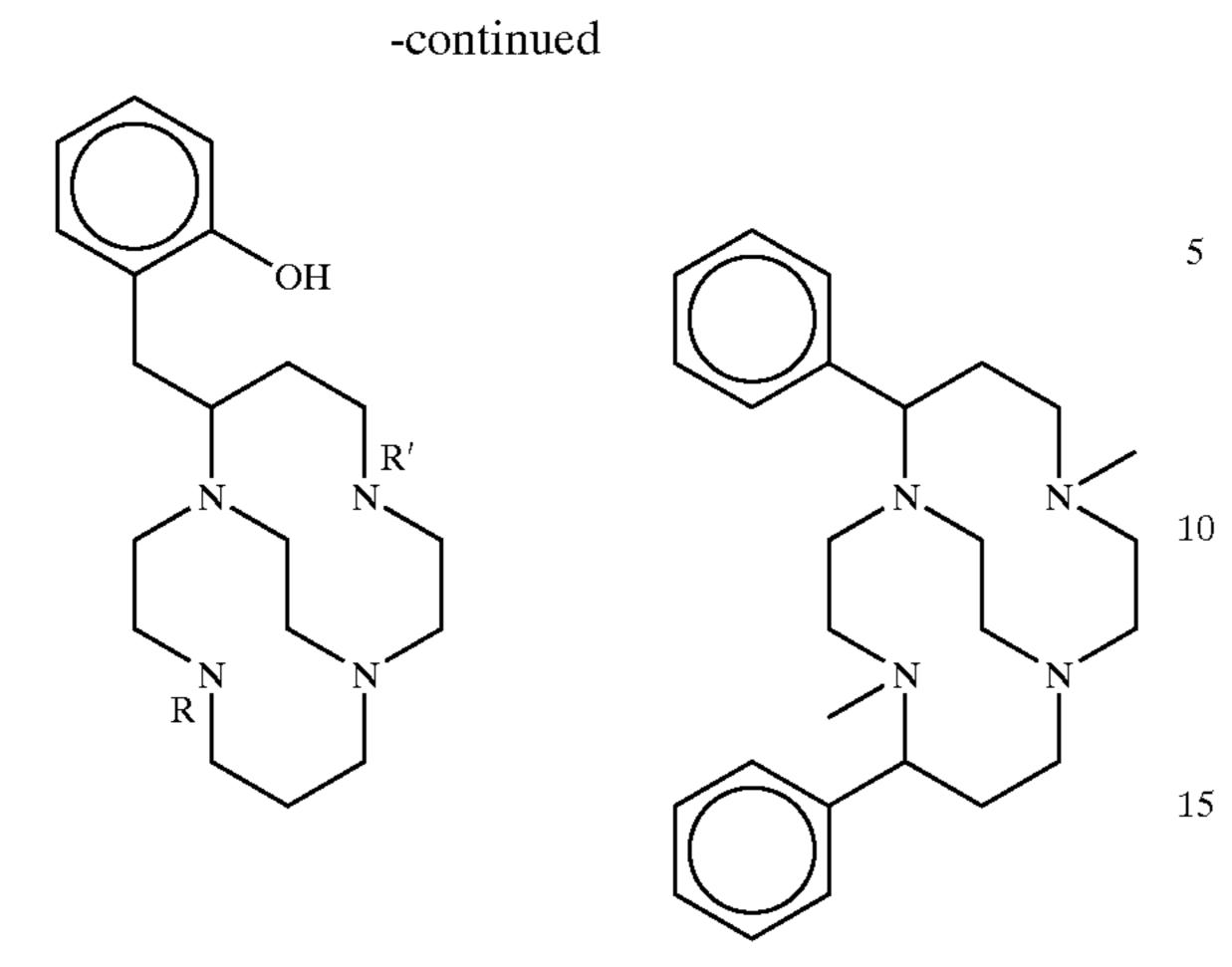
In the above, the R, R', R", R" moieties can, for example, 35 be methyl, ethyl or propyl. (Note that in the above formalism, the short straight strokes attached to certain N atoms are an alternate representation for a methyl group).
