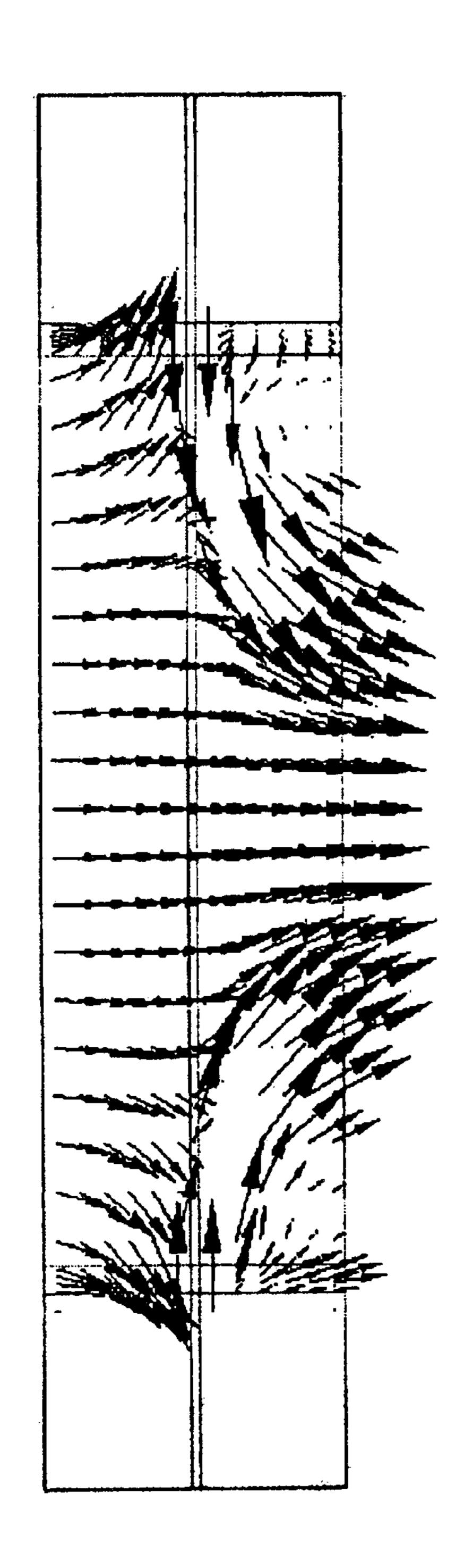
Air injection to stator and movable unit
