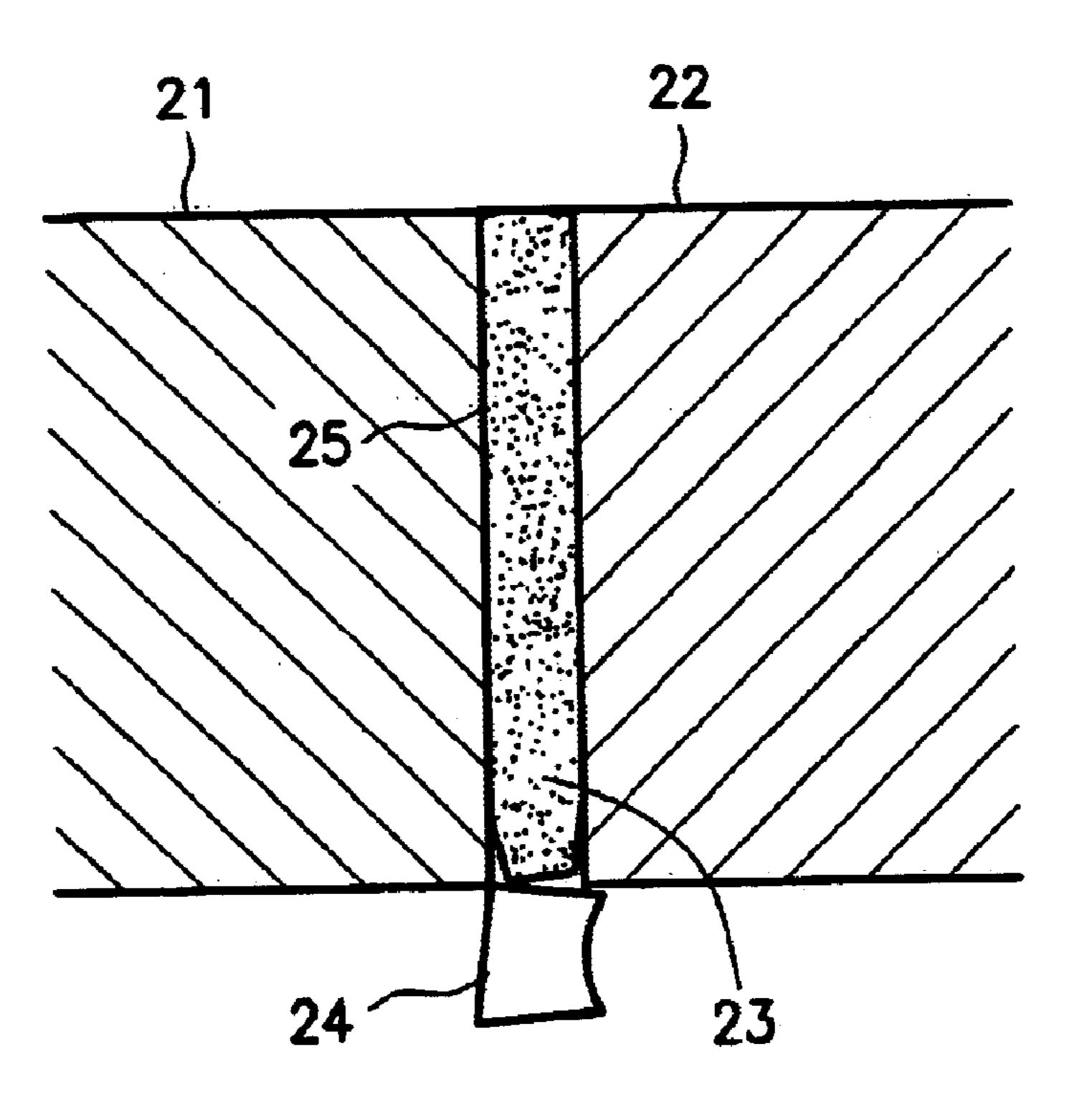
disposing a transmitter for emitting mechanical vibrations in a region of an adhesive join between the components so that the vibrations act upon the adhesive
