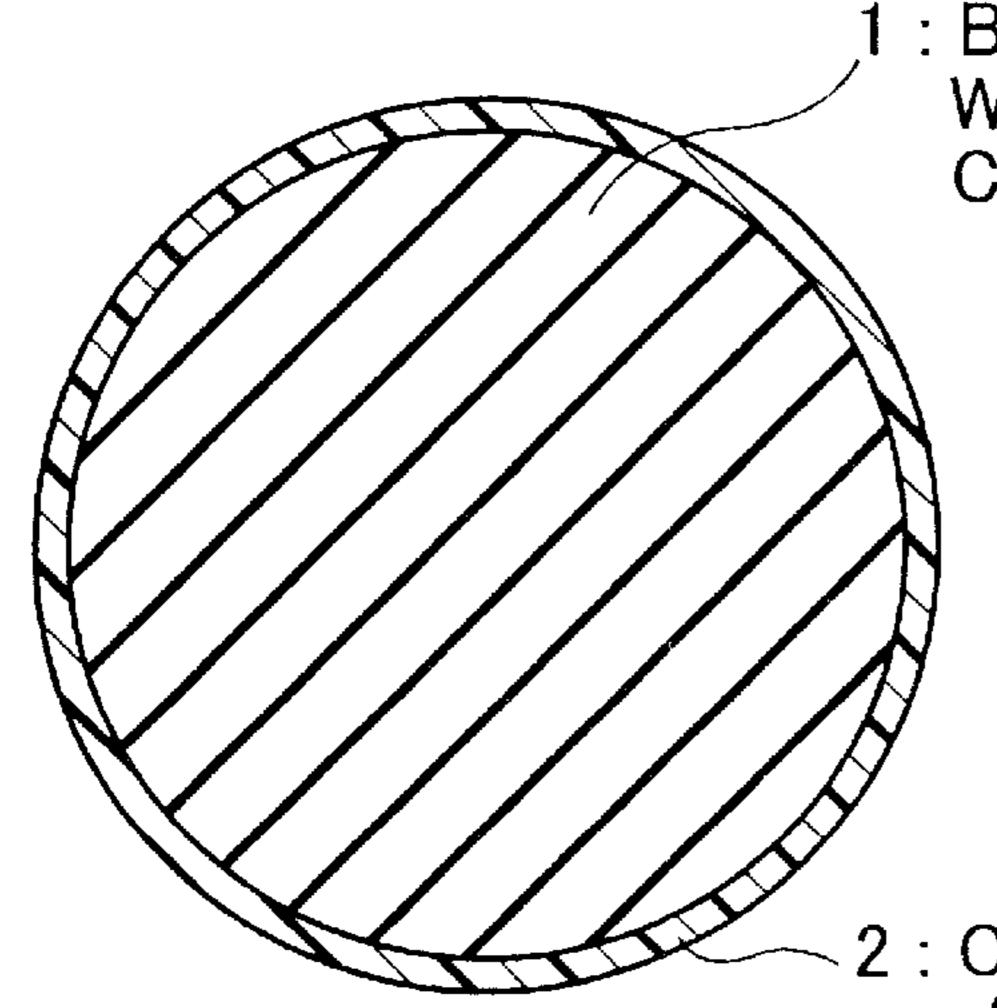
1 : BALL BODY MADE FROM WHITE RUBBER COMPOSITION CONTAINING TIO2 AND BLUE PIGMENT
