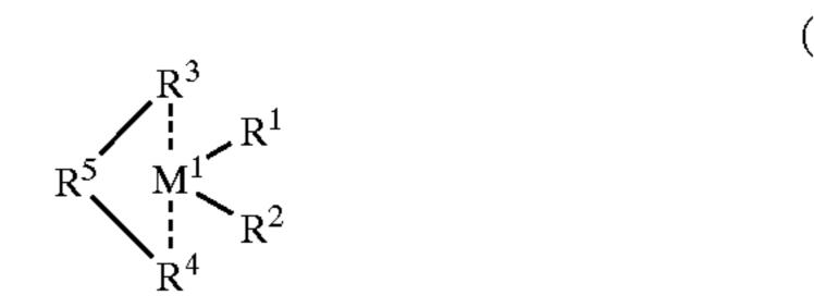
in which M<sup>1</sup> is titanium, zirconium, vanadium, niobium or tantalum, and an aluminoxane. This polyolefin has a very high molecular weight, a very narrow molecular weight distribution and a very high syndiotactic index. Shaped articles produced from the polymer are distinguished by a high transparency, flexibility, tear resistance and an excellent surface gloss.
