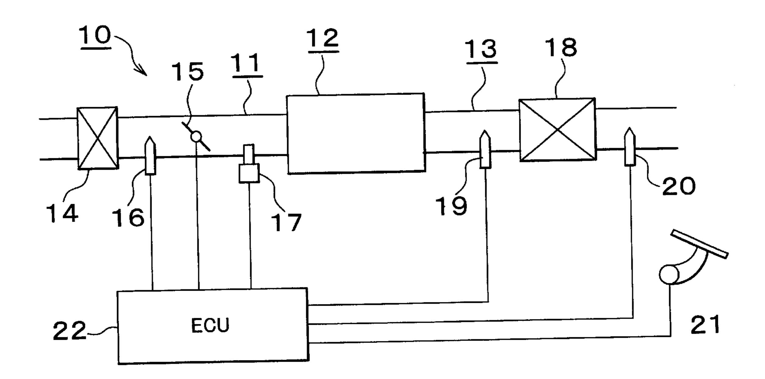
10-INTERNAL COMBUSTION ENGINE 11-INTAKE AIR PASSAGE
