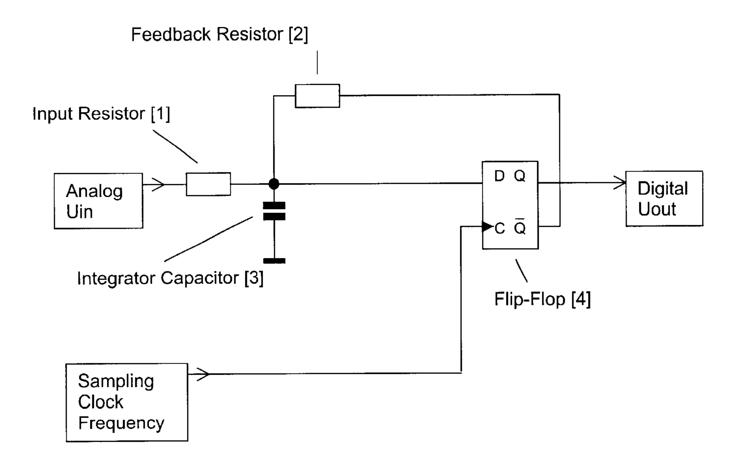
Fig. 2: Improved Delta-Sigma ADC with stabilized and separated power supply for chip internal input and output buffers
