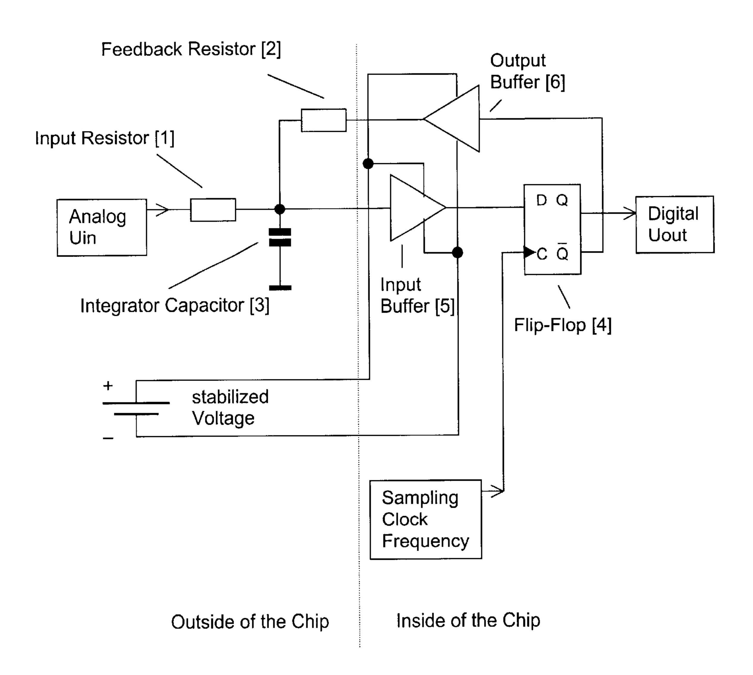
Fig. 3: Improved Delta-Sigma ADC with stabilized separated supply of additional chip external input and output buffers
