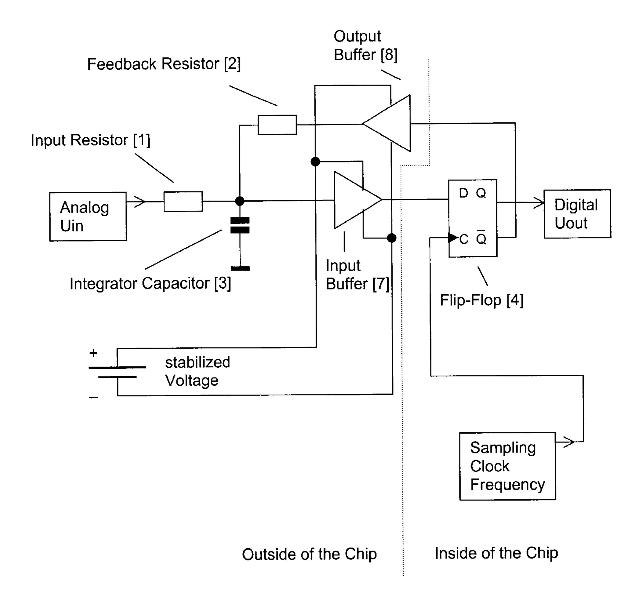
Fig. 4: Sample Scenario for a feed forward leading to a Hysteresis at the input of the Flip-Flop.
