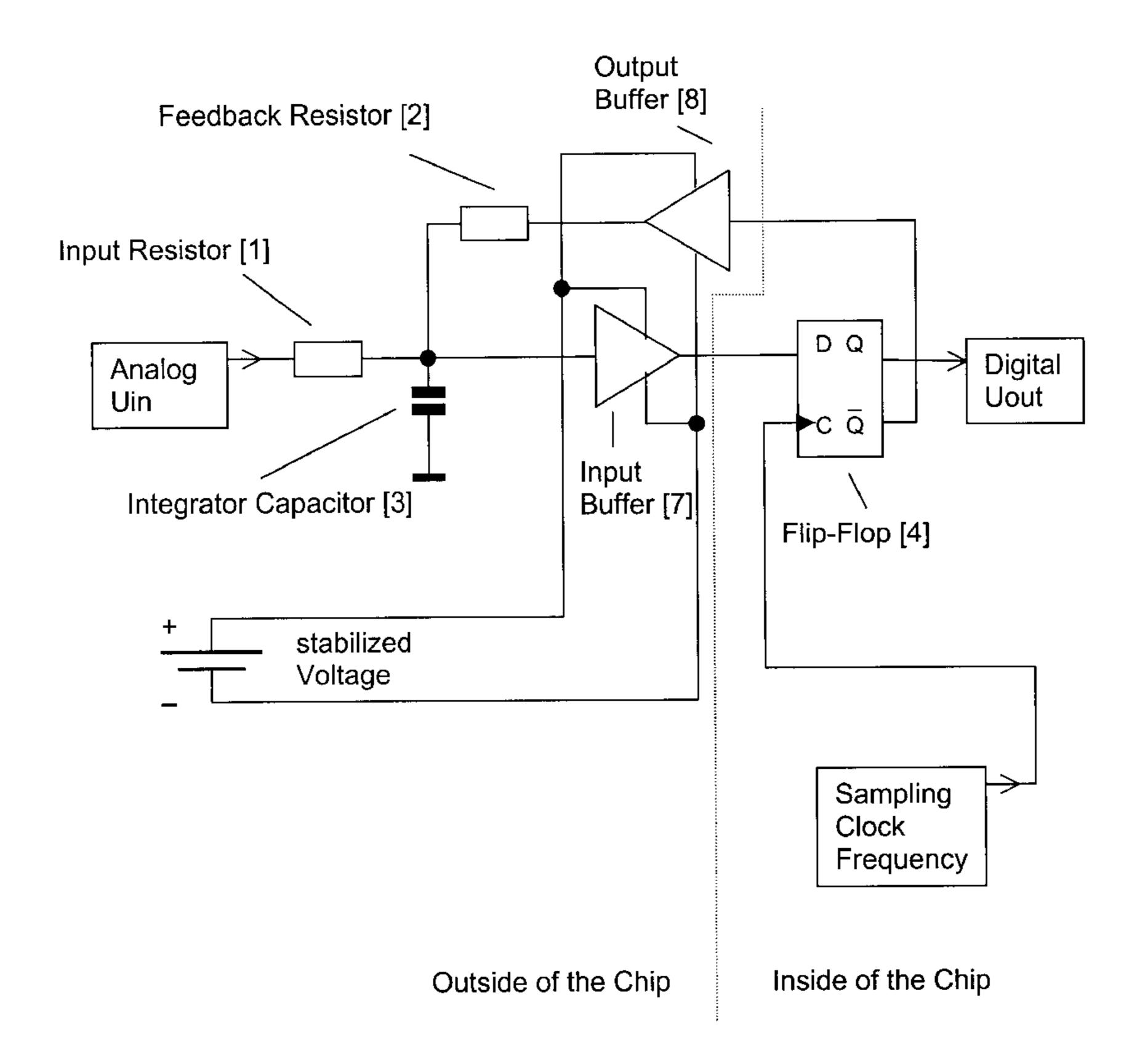
Fig. 1: Simple Delta-Sigma Analog to Digital Converter (prior art)
