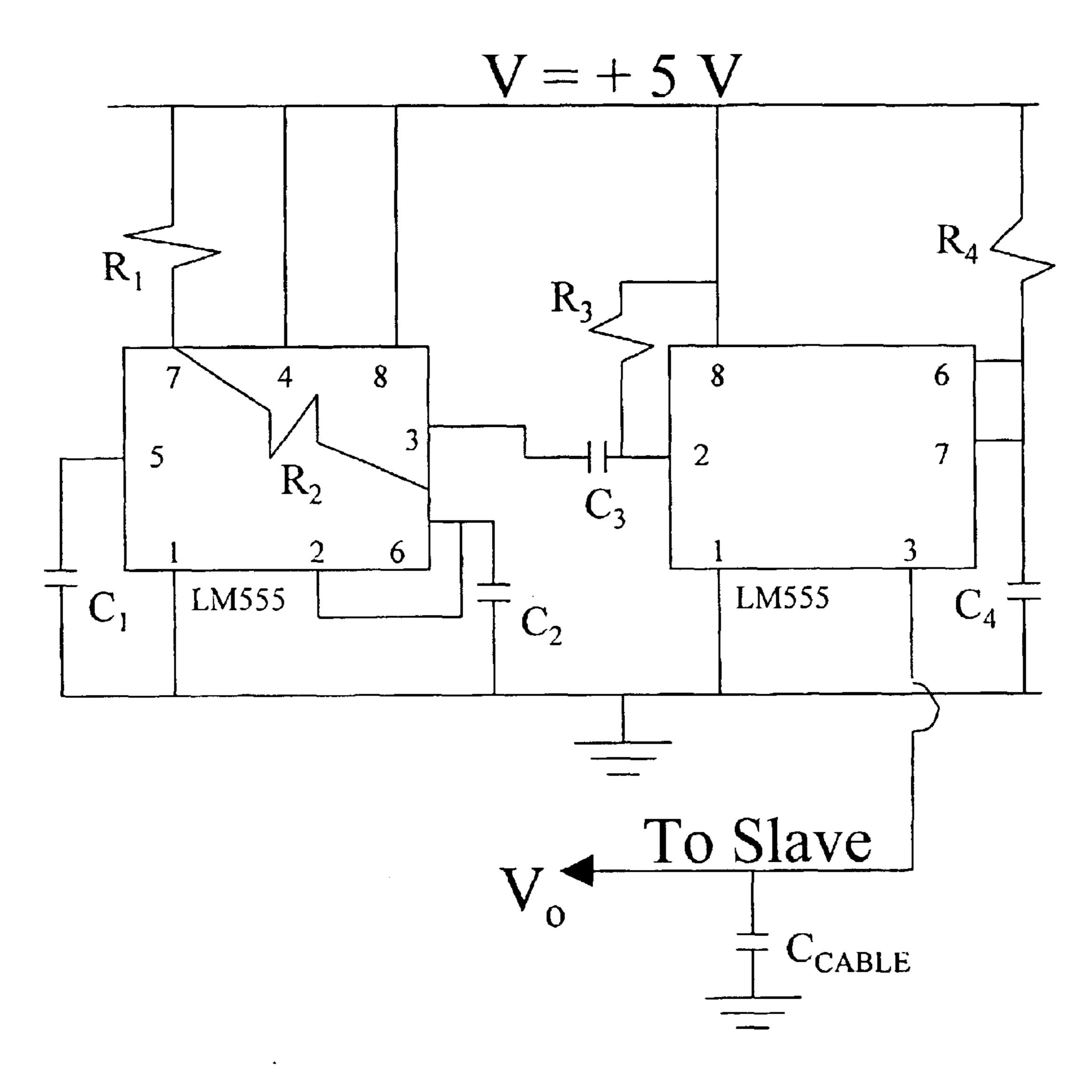
$R_1 = 68 \text{ K}\Omega$   $C_1 = 0.001 \text{ }\mu\text{F}$
