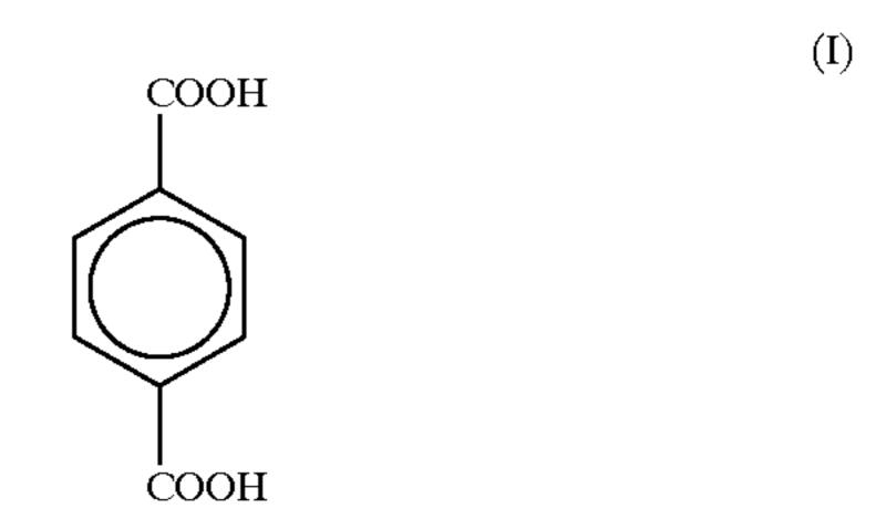
to furning sulfuric acid containing al least 20% of SO<sub>3</sub>, subsequently adding formaldehyde thereinto, heating the mixture at 120-160° C. and isolating the obtained 5-carboxyphthalide.
