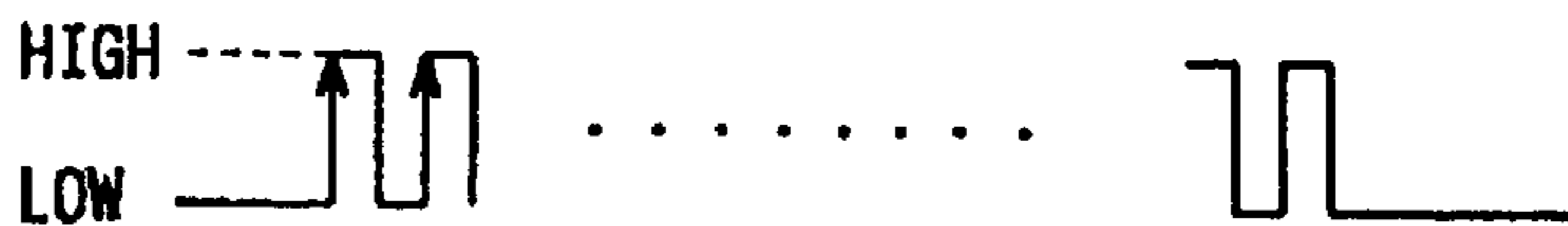
FIG. 8C OUTPUT OF VOLTAGE COMPARATOR (113)
