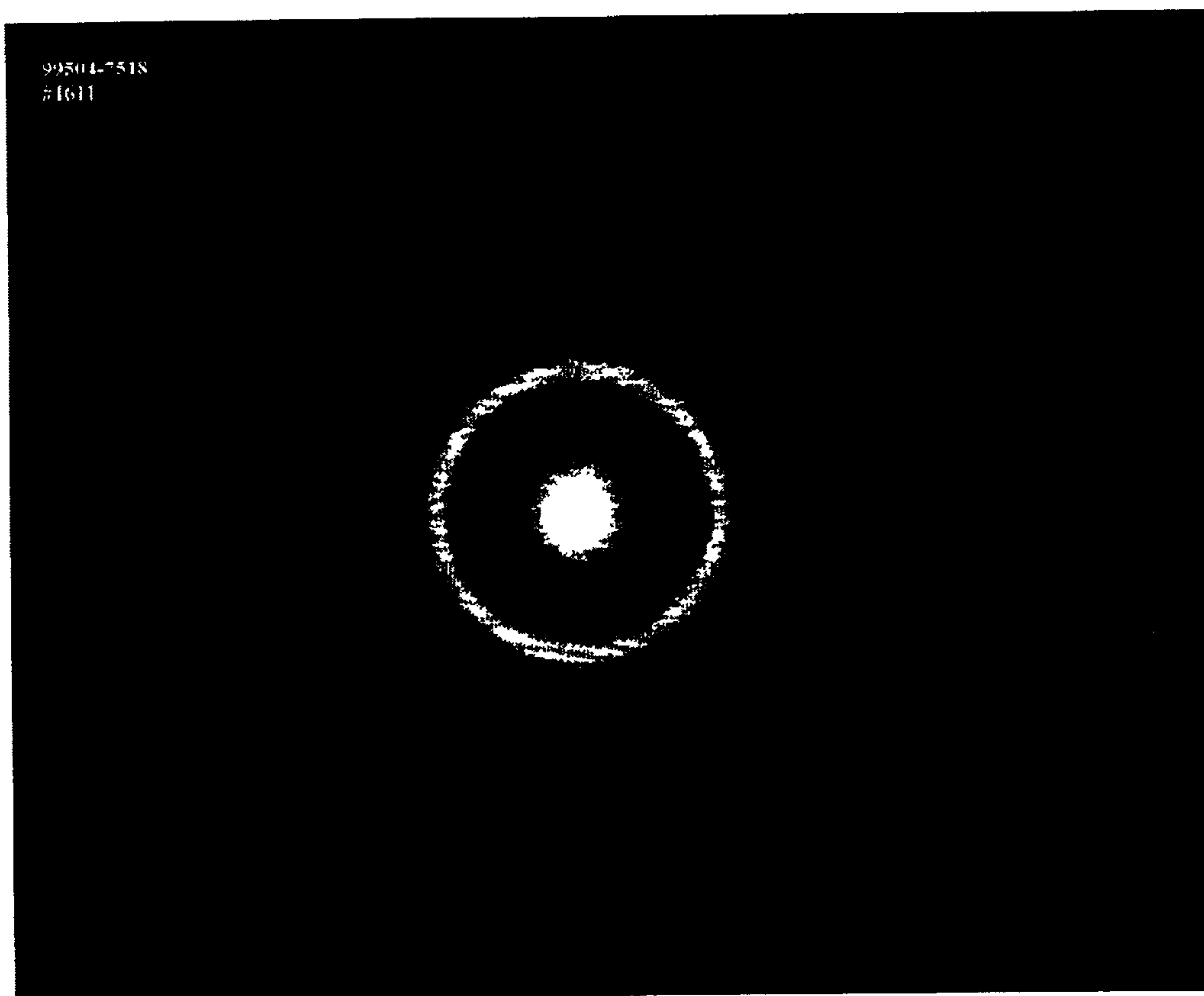
Fig. 6: TEM diffraction pattern of 400Å NiNb films deposited on glass substrates.
