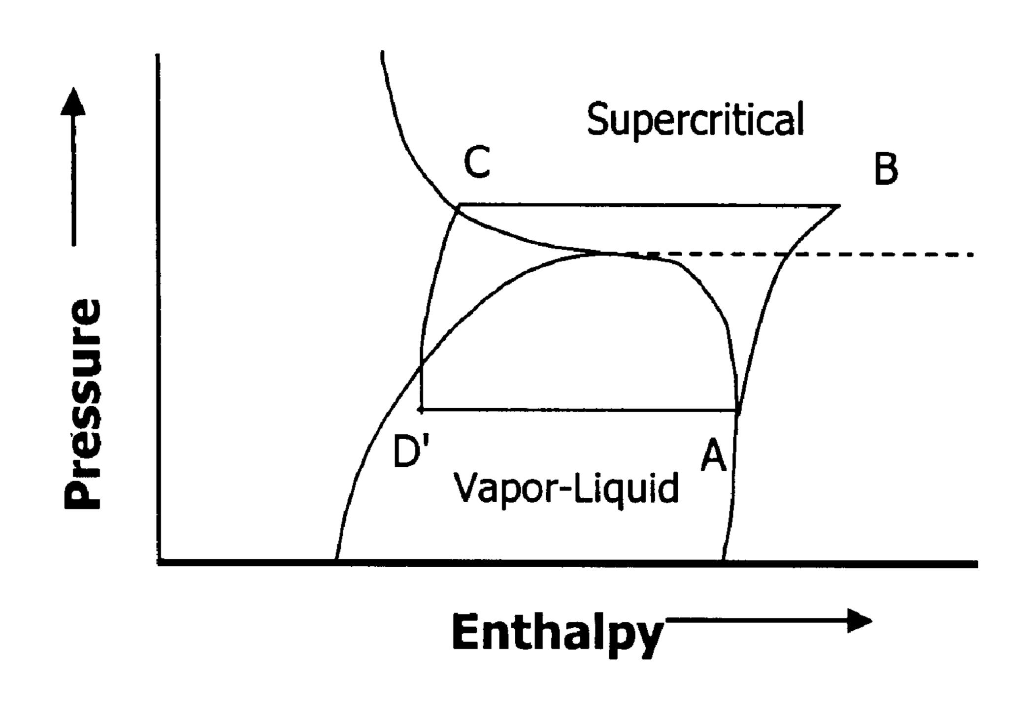
Fig 1. Standard Transcritical Vapor Compression Cycle (Prior Art)
