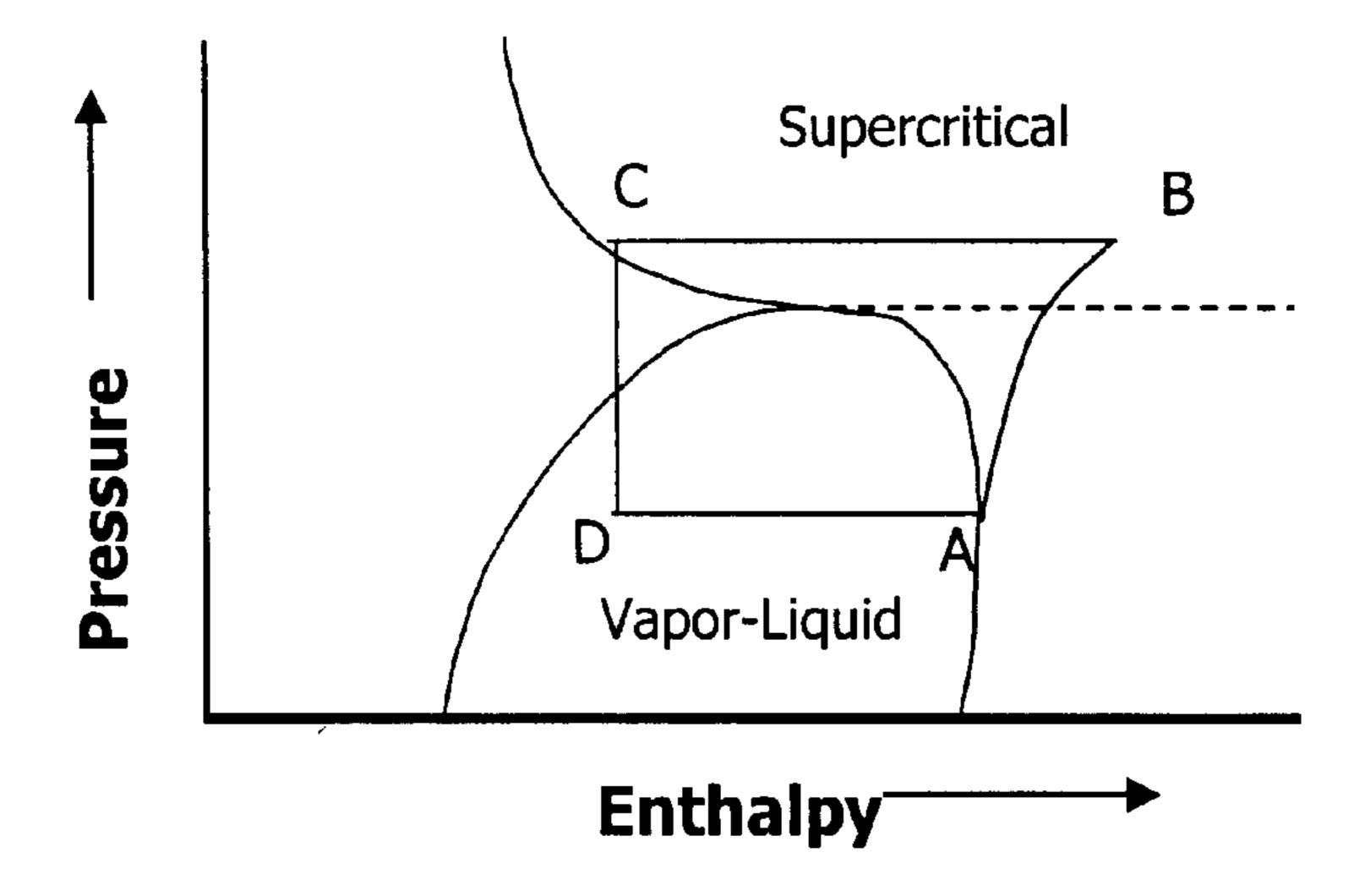
Fig 2. Components for Standard Transcritical Vapor Compression Cycle
