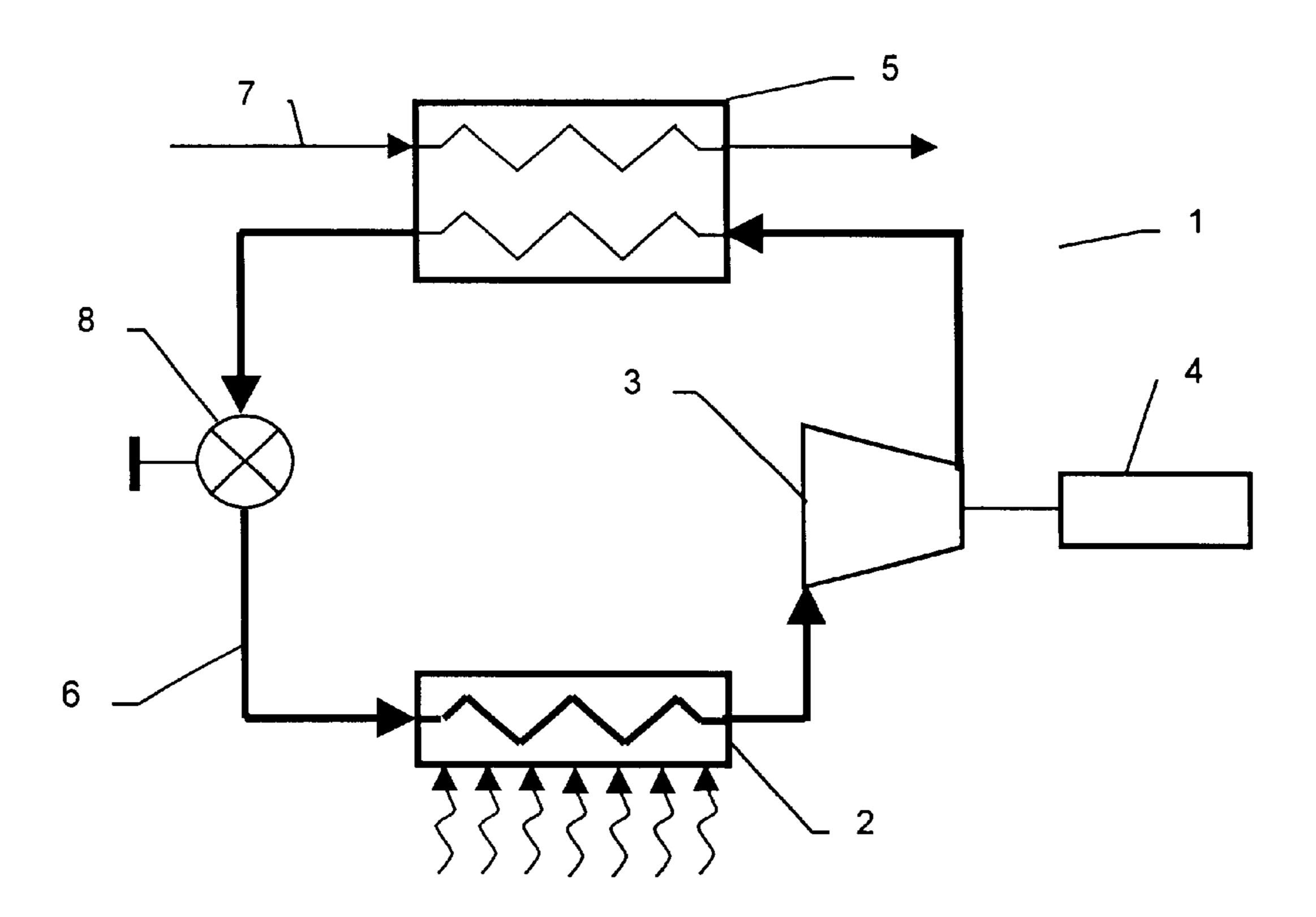
Fig 3. Vapor Compression Transcritical Cycle with Turbine
