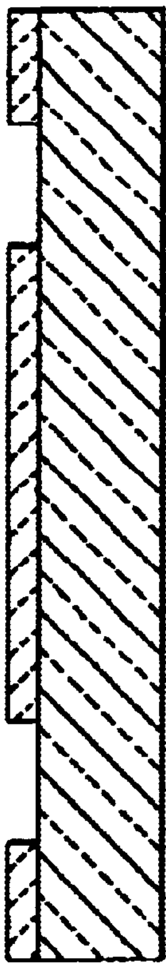
Spin resist on glass slide and expose with mask 4
