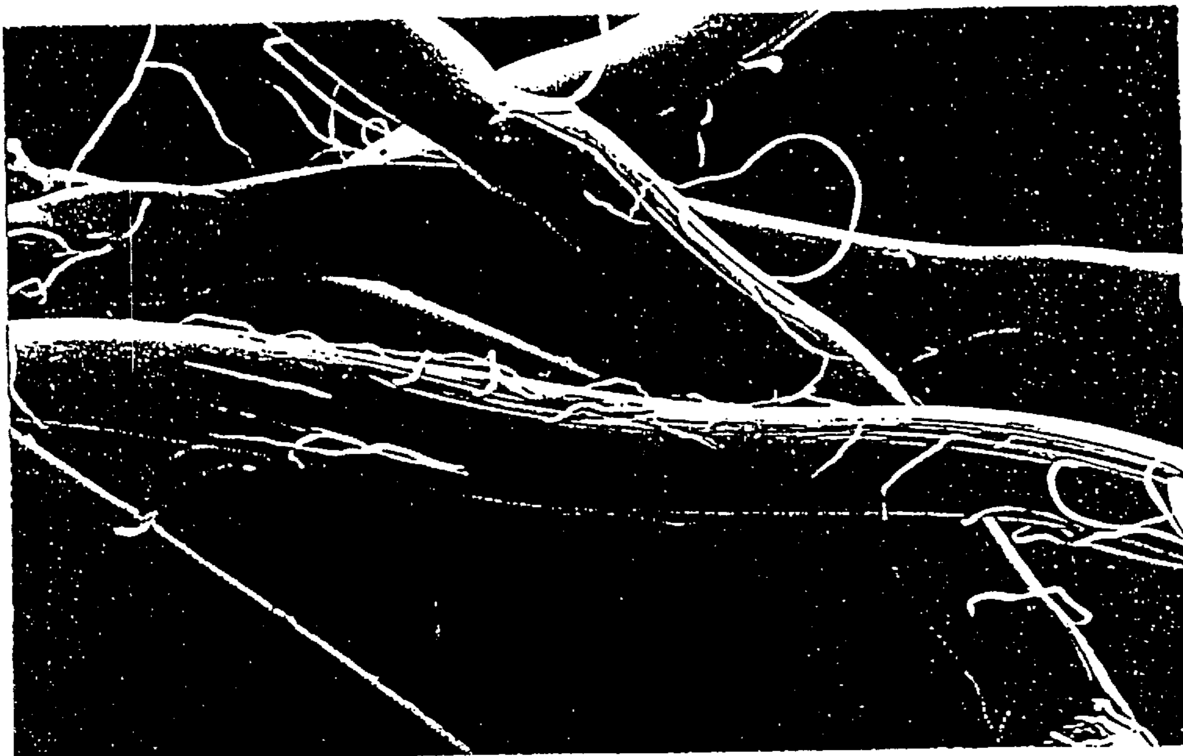
Abraded Commercial Fiber 1 - 1000X
